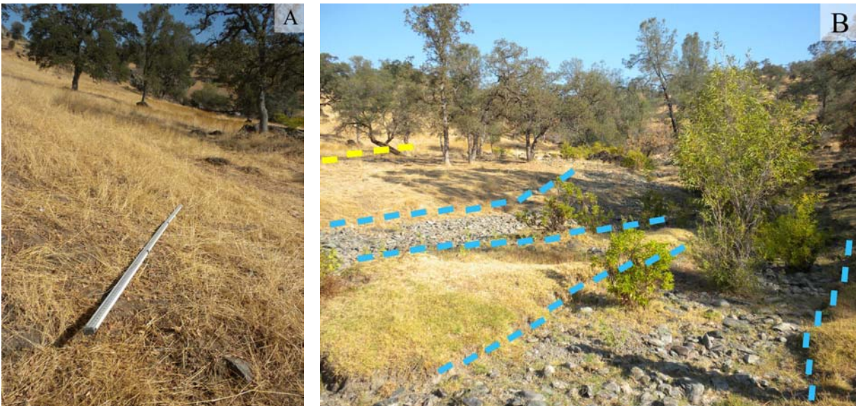
Figure 37. Channel characteristics at Black Creek: (A) gage-predicted OHWM, and (B) field OHWM signature shown by the blue dashed lines. The approximate location of the outer bank of the gage-predicted OHWM is shown by a yellow line in the background and aligns with the extent of the stadia rod shown in A.
