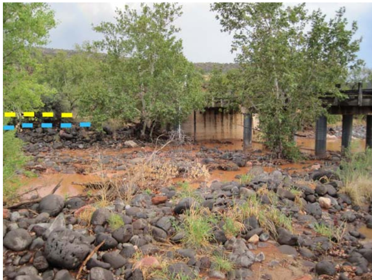
Figure 36. Channel characteristics at Dry Beaver Creek: The field OHWM is shown by the blue dashed line, and the gage-predicted OHWM from the 5.4-year flood in 2007 is shown by the yellow dashed line.
