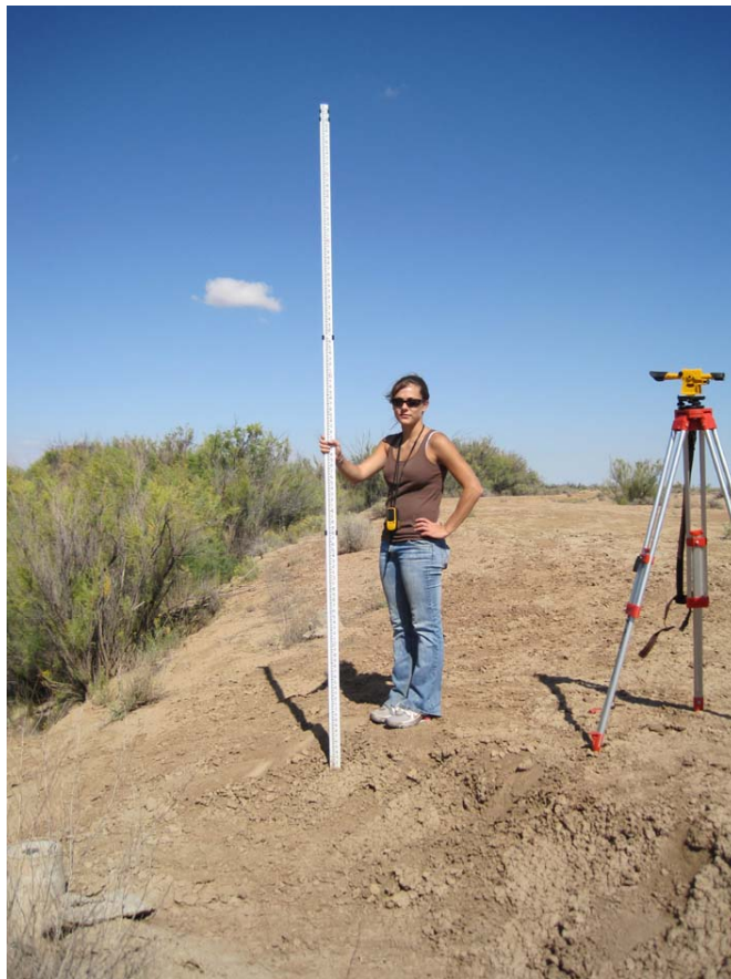
Figure 16. Level and stadia rod used to determine the stage of the field OHWM and the position on the channel bank of the gage-predicted OHWM.
