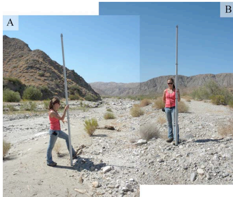
Figure 24. OHWM at Mission Creek: (A) field OHWM shown by the break in slope, change in sediment texture, and change in vegetation successional stage, and (B) gage-predicted OHWM with no indicator changes.
