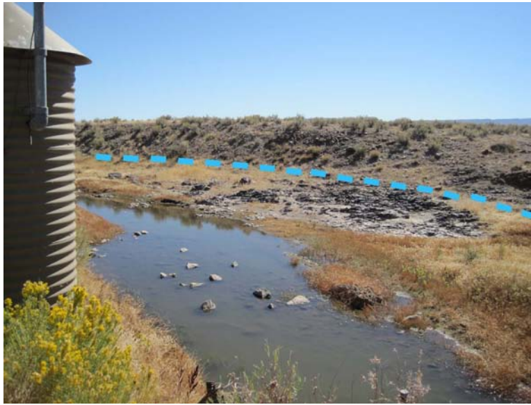
Figure 39. Rock Creek, with the field OHWM shown by the blue dashed line. The field OHWM is located where the bank slope becomes steeper and the vegetation changes.
