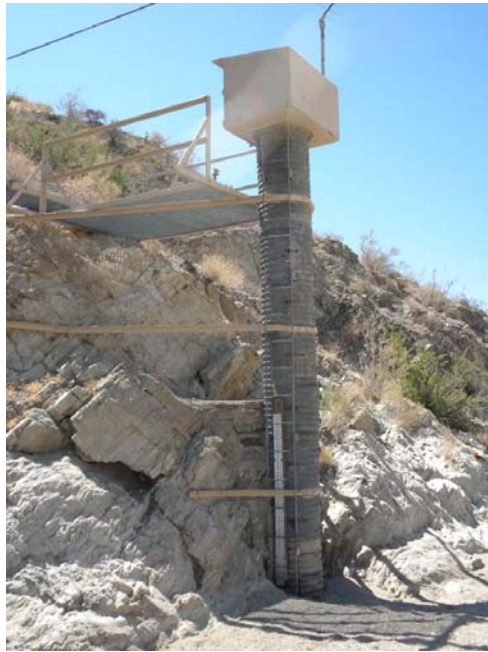
Figure 7. USGS gage with a staff outside the gage. The staff shows the height of the water surface used in developing the stage-discharge relationship.
