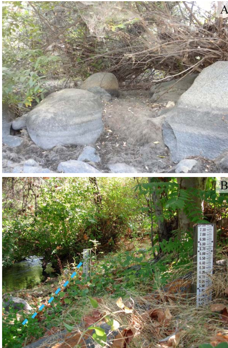
Figure 38. Deer Creek, with the field OHWM shown by the blue dashed line: (A) Active channel. The water line visible on the rocks is common to many of the boulders in this channel. (B) Established vegetation on the slope above the OHWM. The boulders shown in A are covered in this view by water.
