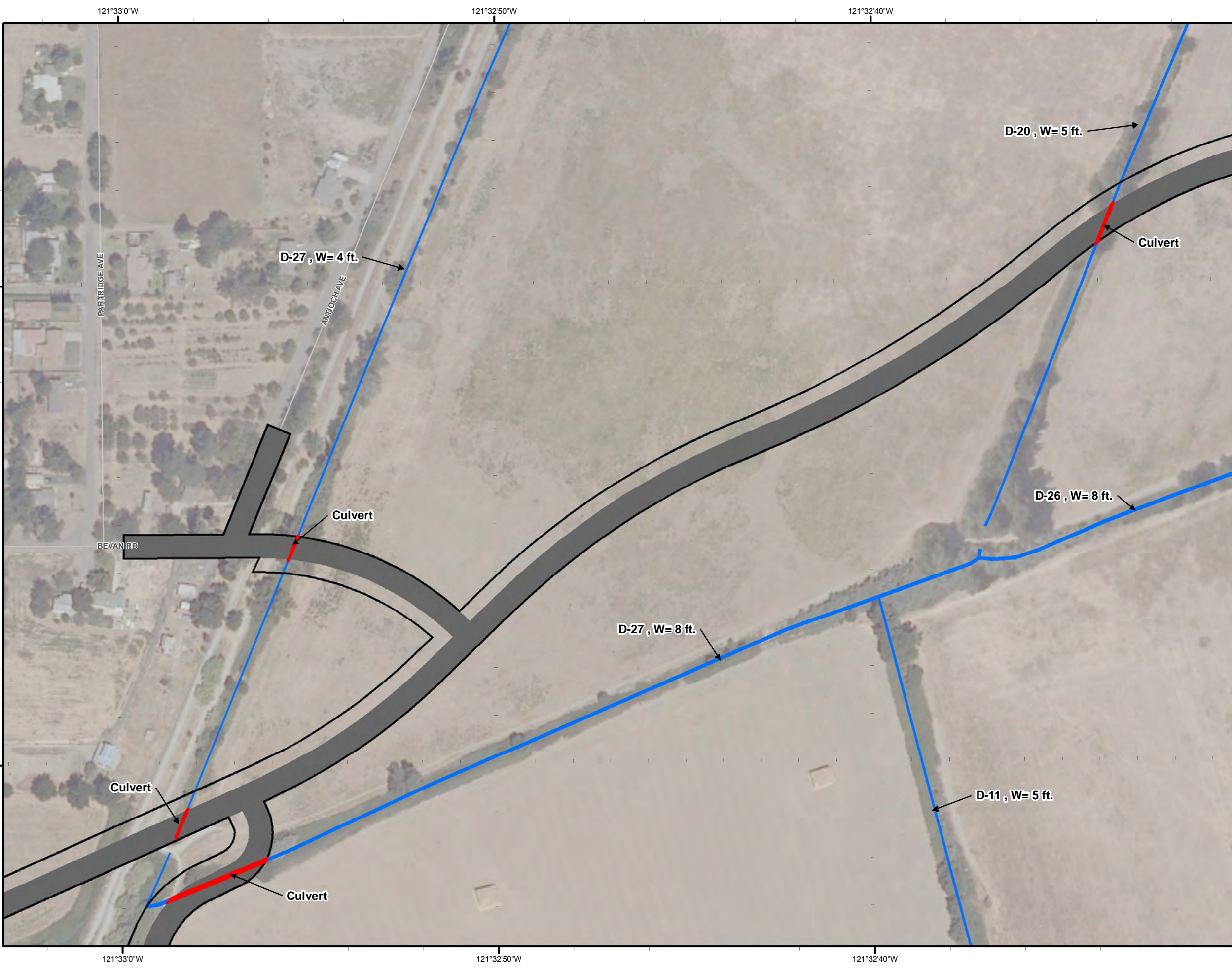
Figure 3 Project Plan View Showing Impacts to Potential Waters of the United States, Including Wetlands
