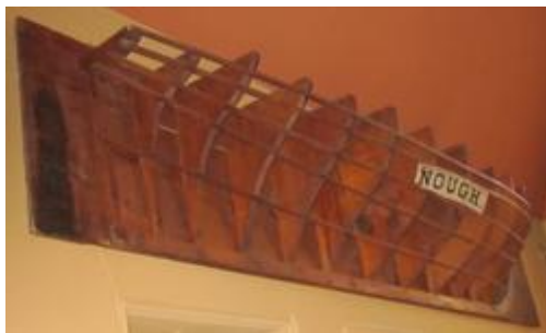
The original half hull "hawk's nest" ship model, used for MacDonough 's construction at Caleb Carr's Warren shipyard in 1815.
