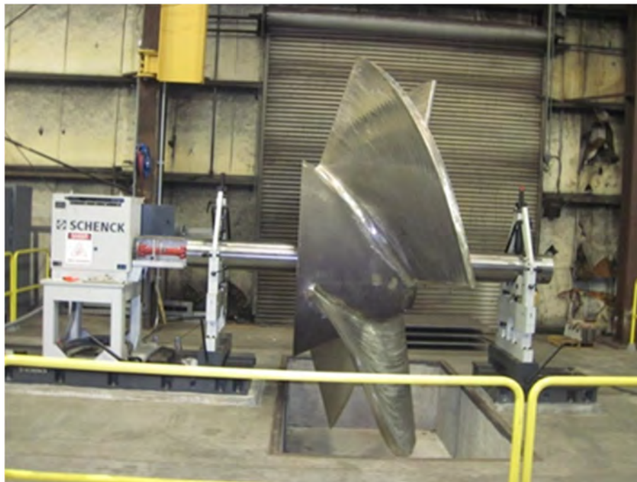
Figure 10.2. Impeller Balancing Machine for Two Plane Balancing
