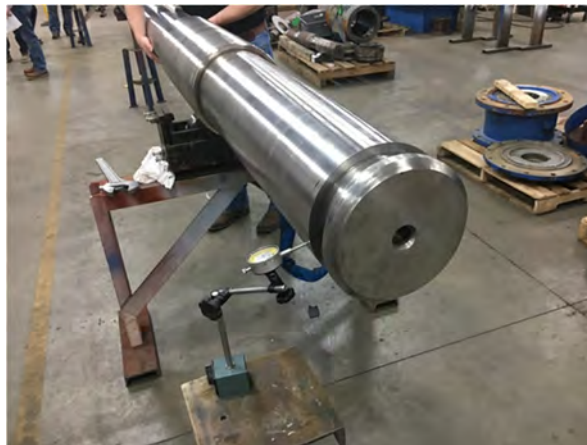
Figure 10.6. Checking Shaft TIR/Runout with Dial Indicator
