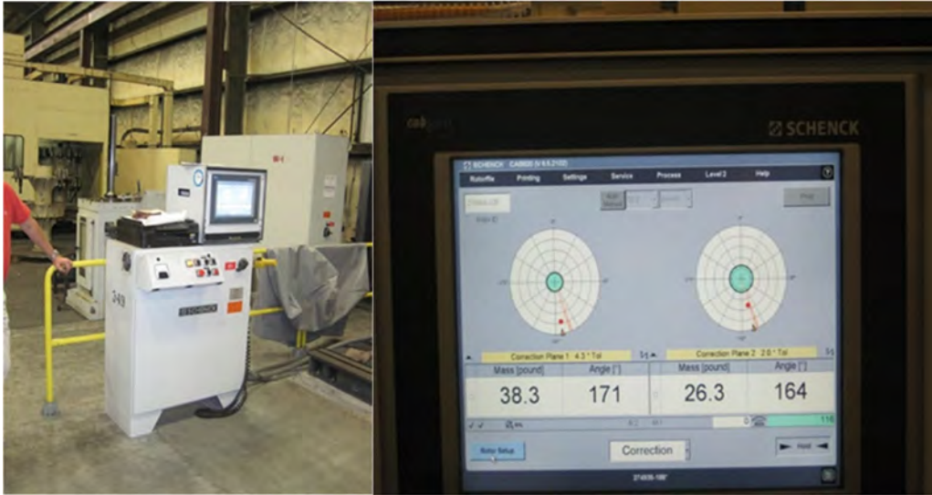
Figure 10.3. Correction Information that is obtained for Two Plane Balancing
