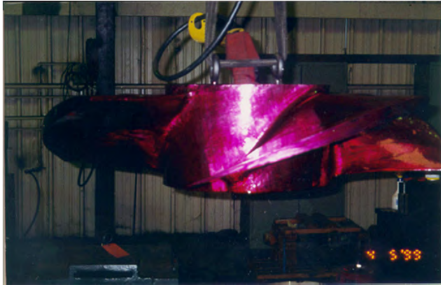
Figure 10.7. 1 st Stage Dye Penetrant Non-Destructive Testing of Impeller for Damage to Casting
