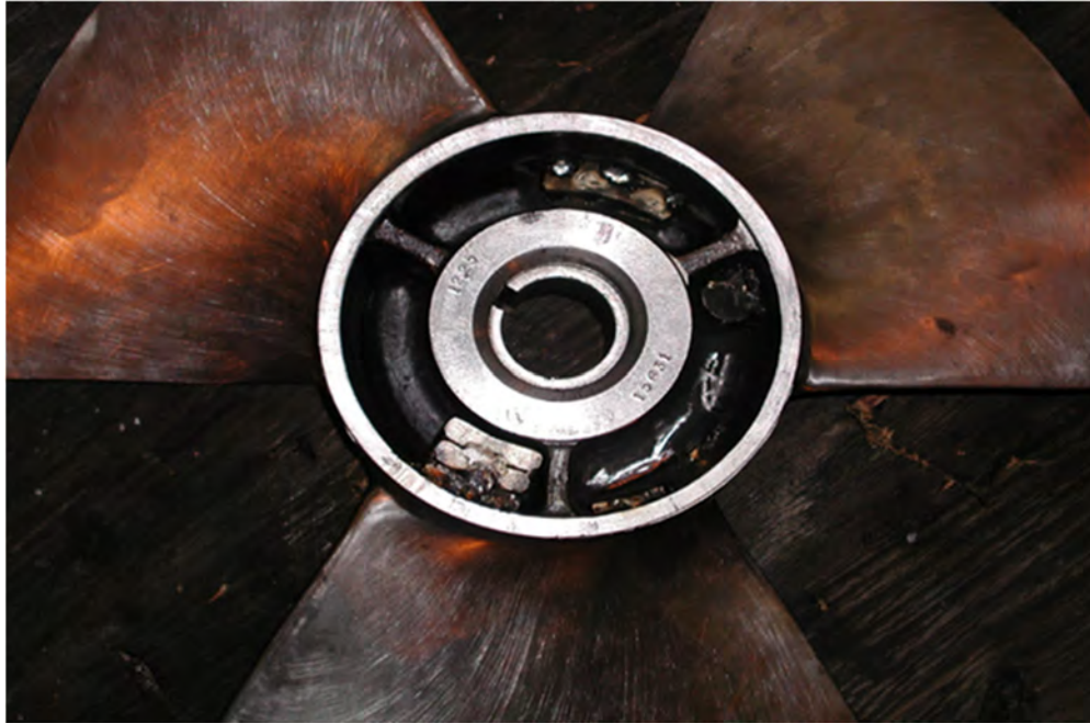
Figure 10.5. Pump impeller with weights and keyway (Note Weight Stamper on Impeller)
