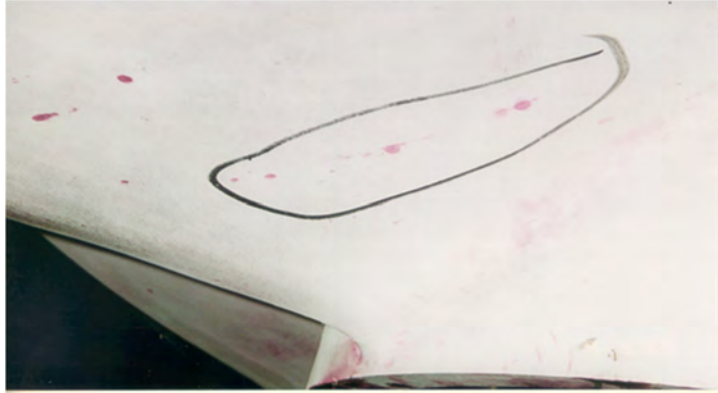
Figure 10.9. Examination of Potential Areas of Cavities Found During Dye Penetrant Testing
