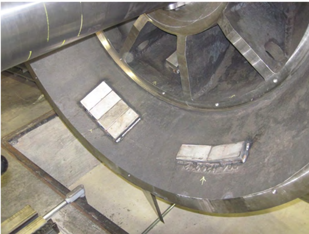
Figure 10.4. Weights Welded to Back of Impeller Out of Water Passage for Two Plane Balancing Corrections
