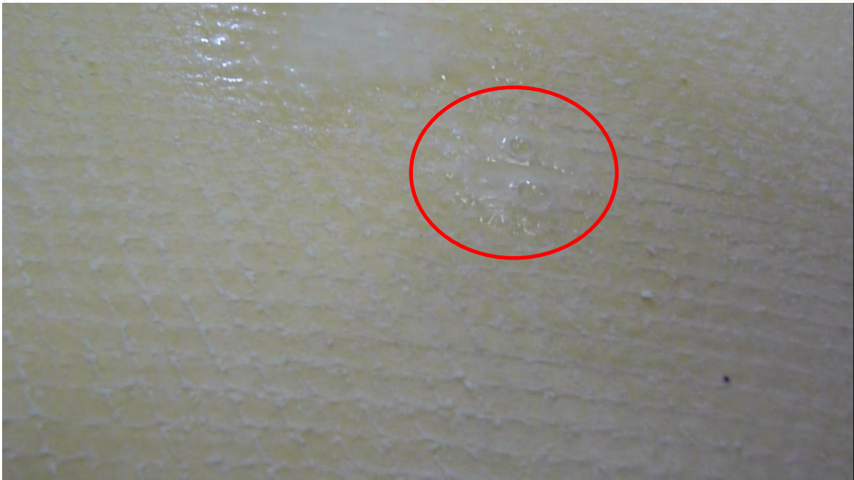
Fig. 1: Precipitants on membrane surface, bubbles in red circuit mean gaseous CO 2
