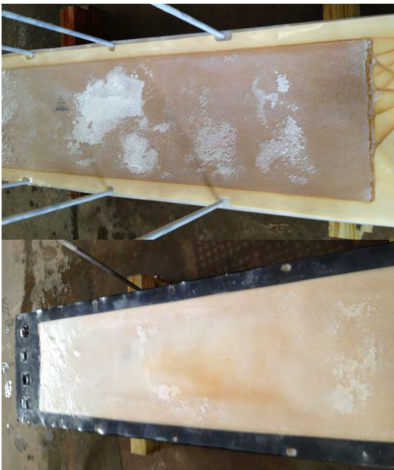
Figure 18.—EDM-2 center membrane (top) and center divider (bottom).
