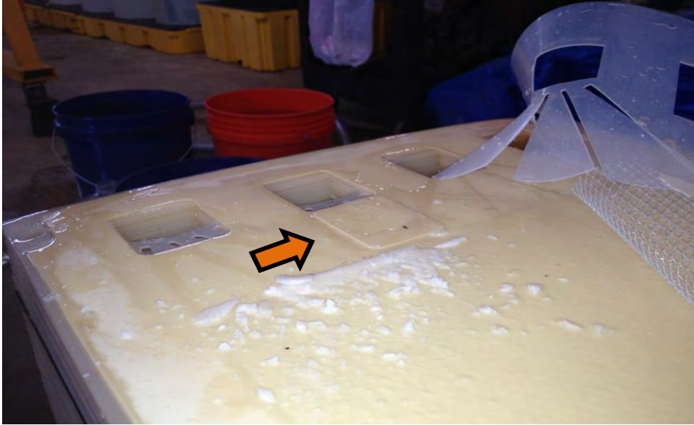
Figure 17.—EDM-1 Stack with membrane piece from manufacturer.
