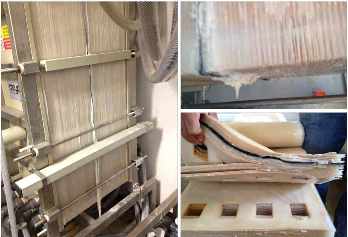
Figure 25.—EDM-2 precipitation and damage from mixing at center of stack.
