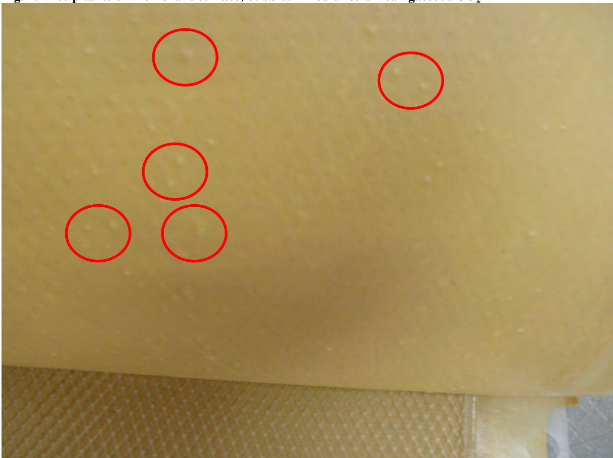
Fig. 2: Precipitants inside membrane
