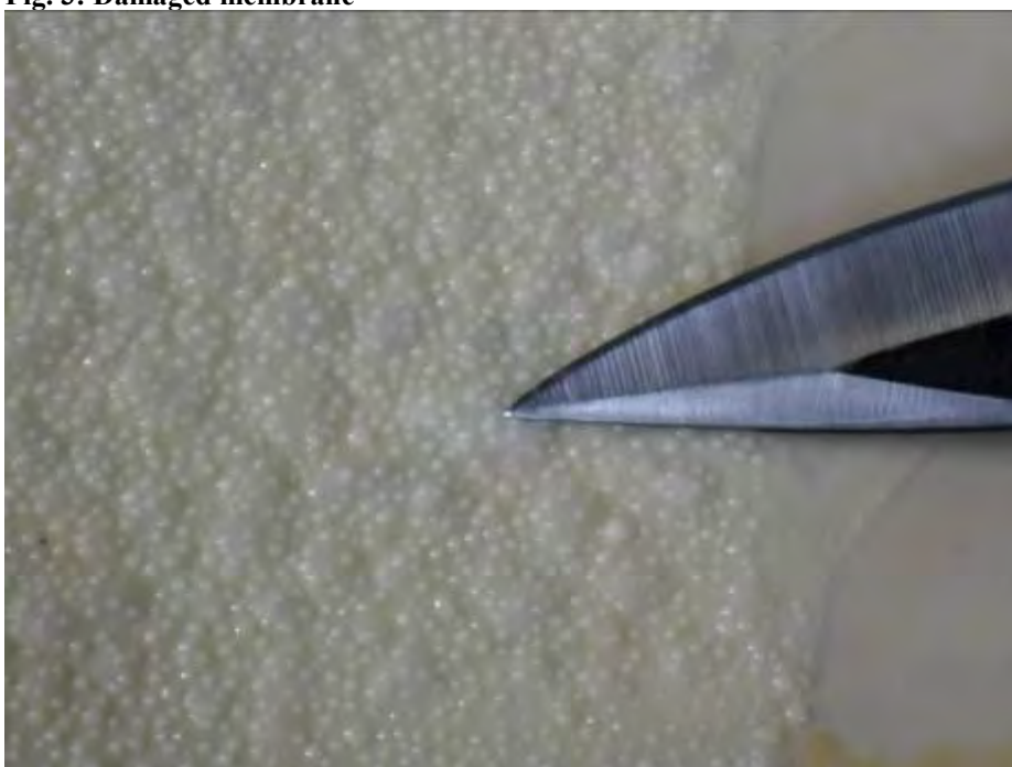
Fig. 4: Precipitants of CaF 2 inside membrane
