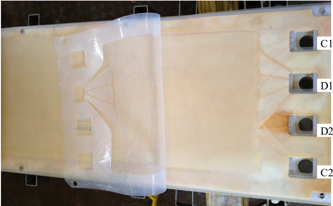
Figure 16.—EDM-2 Stack with corrected D1 (NaCl outlet) spacer installation.
