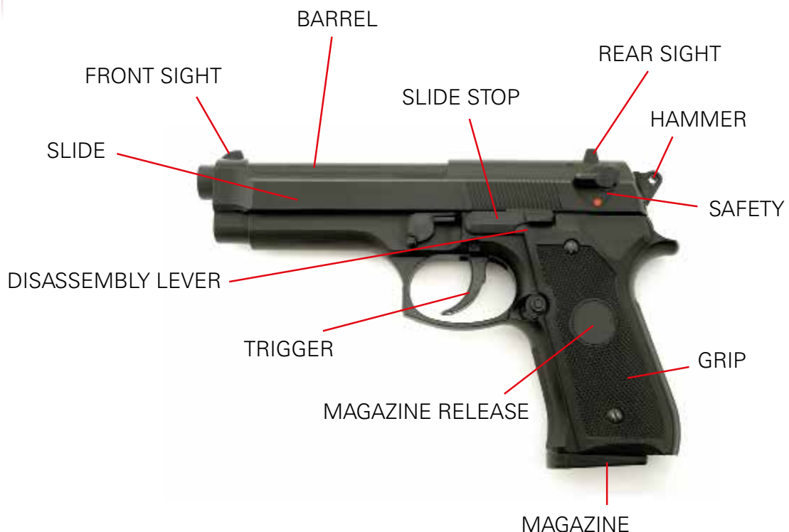
Fig. 22 Parts and components of a pistol
