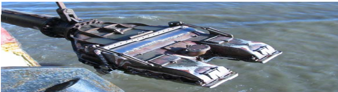
Dredging is accomplished by a drag arm on each side of the ship with a drag head at each end. As the ship navigates the channel with its dredging pumps engaged, the drag heads are lowered to the channel bottom. Like vacuum cleaners, they pull the dredged material into the ship's hoppers.
