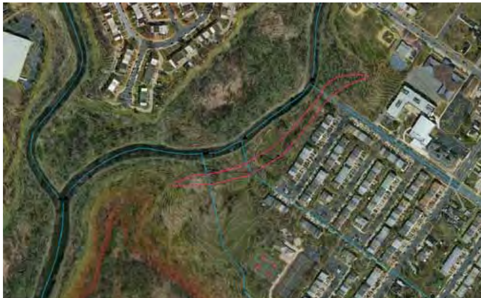
The Eastwick neighborhood is located at the confluence of Darby and Cobbs Creeks in Southwest Philadelphia. USACE developed a hydraulic model to evaluate levee construction as an alternative to protect the Eastwick neighborhood from flooding.
