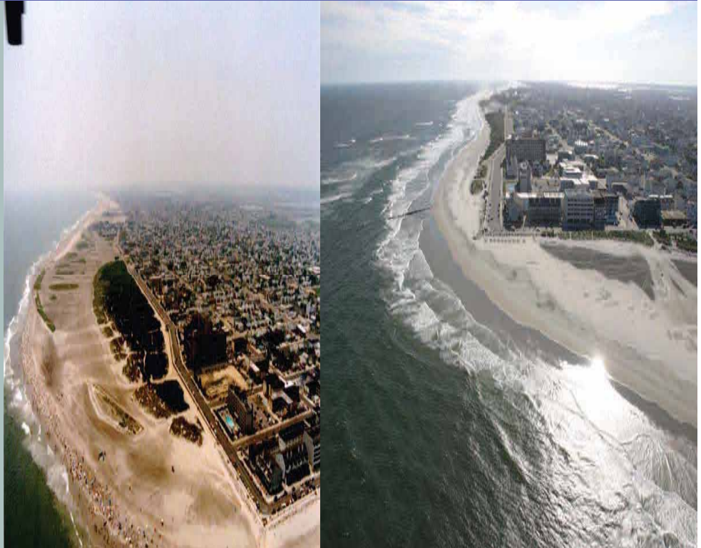
The photo to the left shows the extent of the North Wildwood Beach from July 1989. The photo to the right from 2004 of the same area demonstrates the extent of the erosion that has taken place since 1989.
