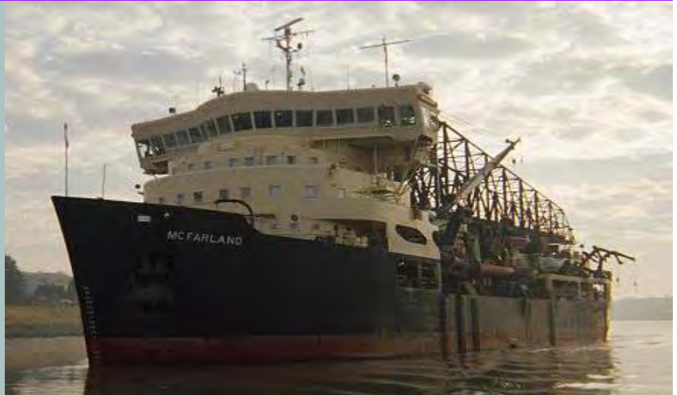
One of four oceangoing hopper dredges owned and operated by the U.S. Army Corps of Engineers as part the Corps' "minimum fleet" for national security and safe navigation, the McFarland is the only dredge in the world with triple capability for direct pump out, bottom discharge and side casting or boom discharge.
