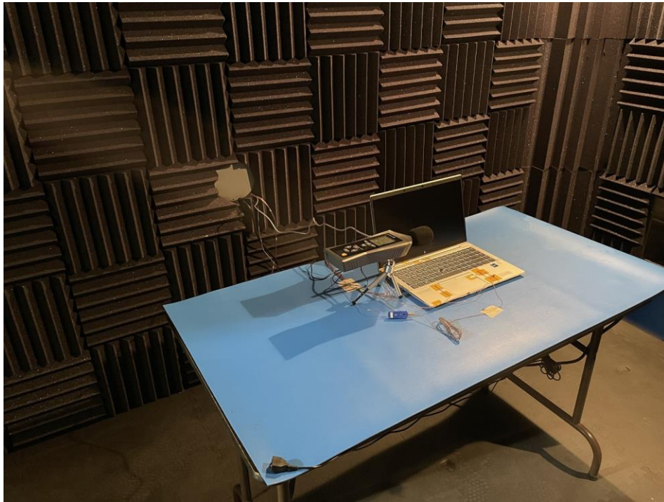
Figure 15. STL pseudo-anechoic chamber testing the HP EliteBook 840 G9
