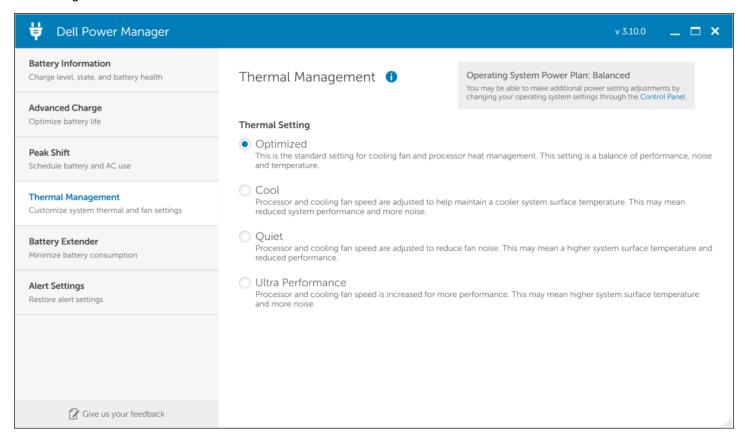
"Optimized" is the default mode that your Dell notebook ships in out of the box. It reflects a balance of all previously established thermal constraints impacting application performance, fan noise, skin temperatures, and battery life.
