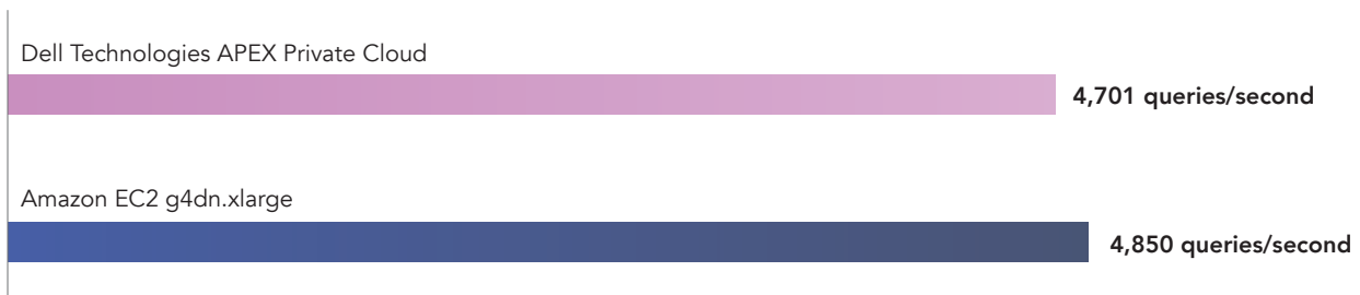
Figure 2: The queries per second that the machine learning VM of the APEX Private Cloud solution and EC2 g4dn.xlarge instance handled during the image classification workload we used in testing. Higher is better. Source: Principled Technologies.
