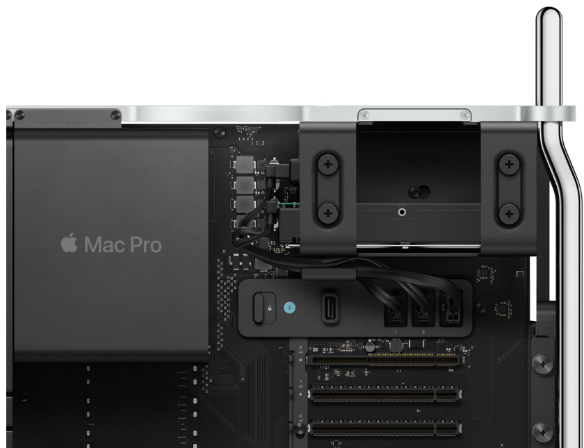
USB 3 and two SATA ports provide internal connectivity for third-party accessories.
