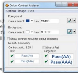
Figure 5: Blue text against a white background provides sufficient contrast, with a luminosity contrast ratio of 9.25:1.
