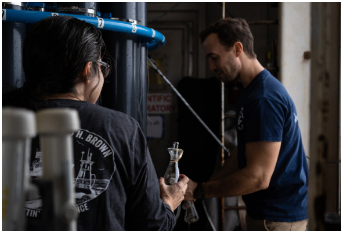
Scientists collect water samples from a CTD cast aboard the R/V Ronald H. Brown during the 2021 PIRATA cruise.
