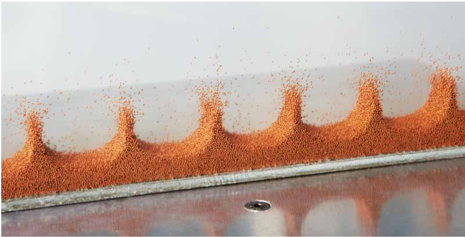
Figure 5: Granular systems: Formation of surface waves in vibrated beds
