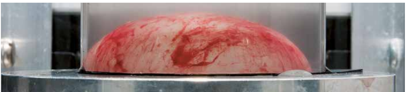
Figure 3: Cyclic inflation experiment on human fetal membrane (diameter 50 mm)
