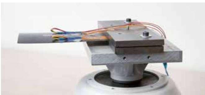
Figure 2: Multi-stable composites with integrate piezo actuators
