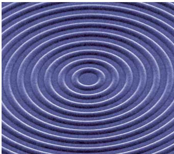
Figure 3: Metallic bull's eye pattern for thermal beaming of a heat ray
