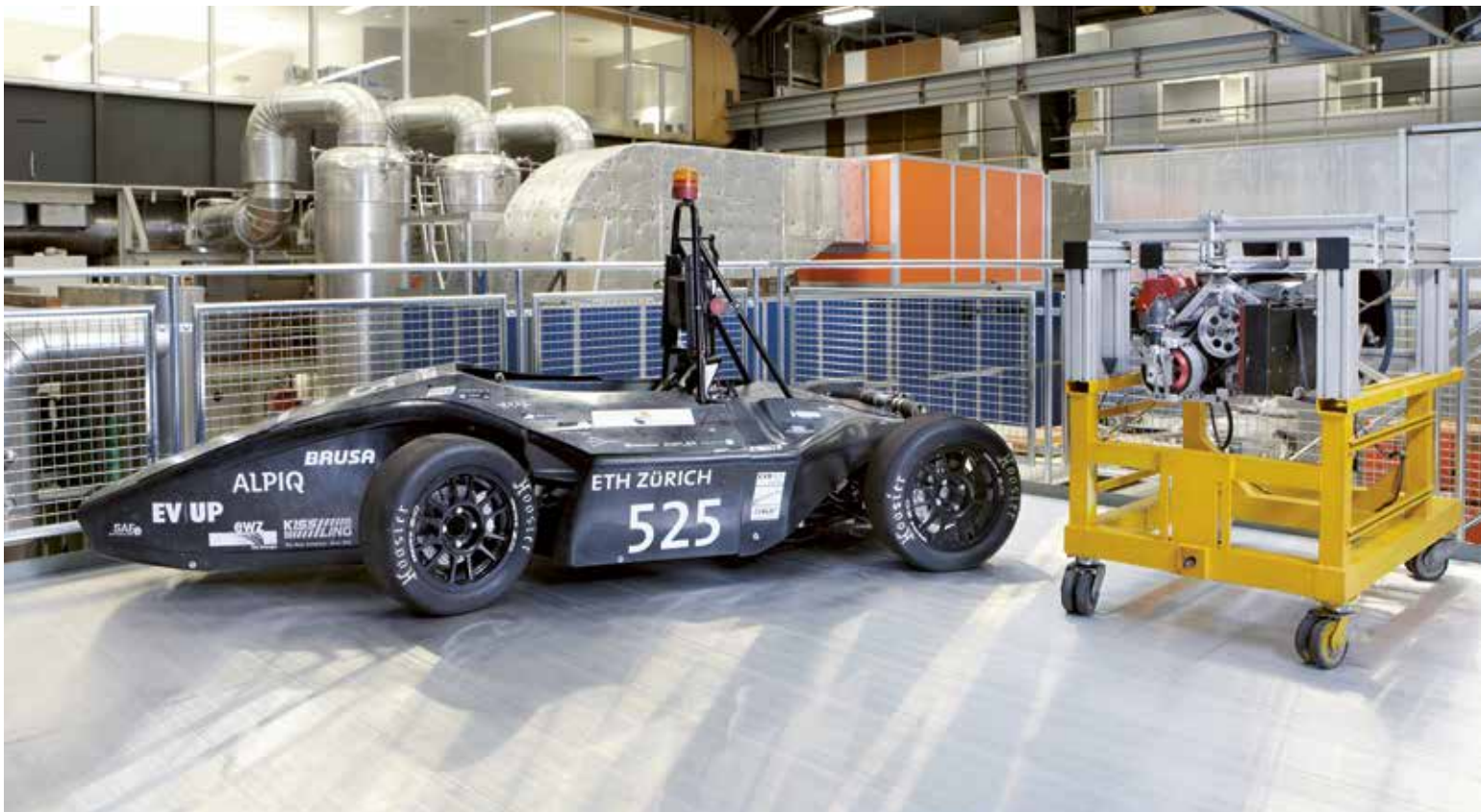
Figure 4: Formula hybrid vehicle and powertrain
