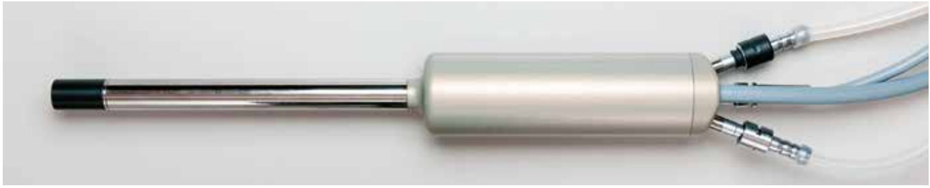
Figure 4: Tissue aspirator for mechanical characterization of the ecto-cervix in pregnancy
