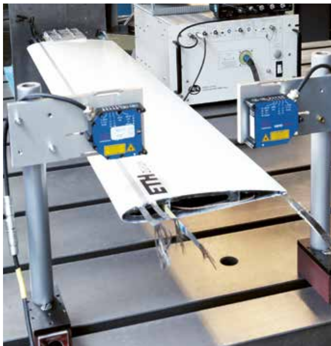
Figure 1: Semi-active airfoil with variable bending/twist-coupling
