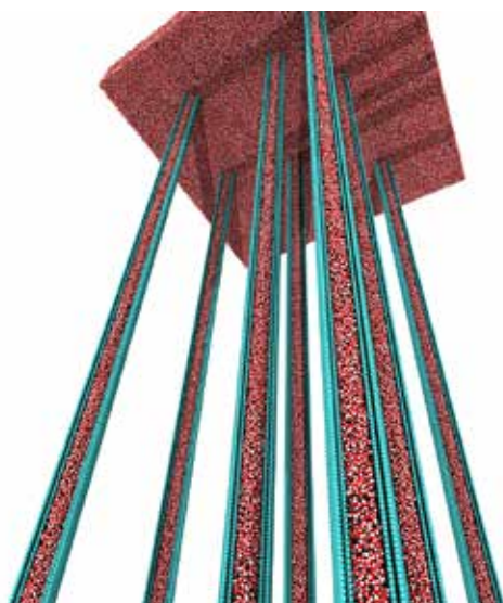
Figure 4: Molecular dynamics simulations of water being transported via micrometer-long carbon nanotube membranes.
