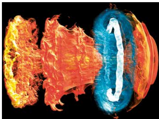
Figure 1: 3D simulations of shock-bubble interaction (density volume rendering)
