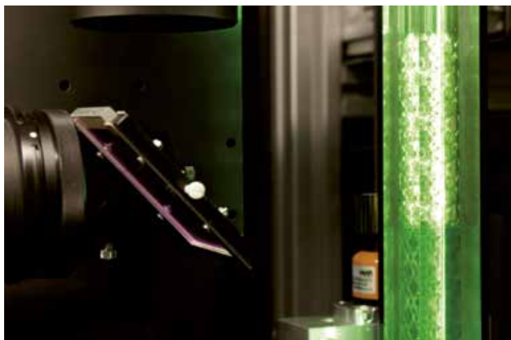
Figure 2: Transparent designed porous structure reactor for the simultaneous investigation by laser induced fluorescence and particle image velocimetry
