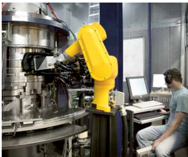
Figure 1: Multi-stage axial turbine research facility with automated robotic arm
