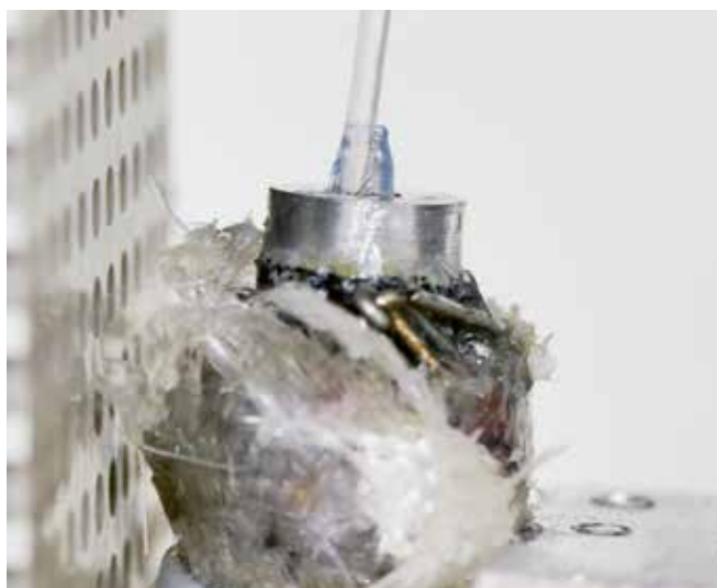
Figure 5: Spider robot that uses thermoplastic adhesives for dragline locomotion (in detail)
