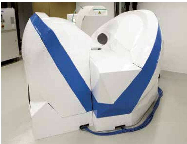
Figure 3: Human-sized magnetic manipulation system with integrated fluoroscope
