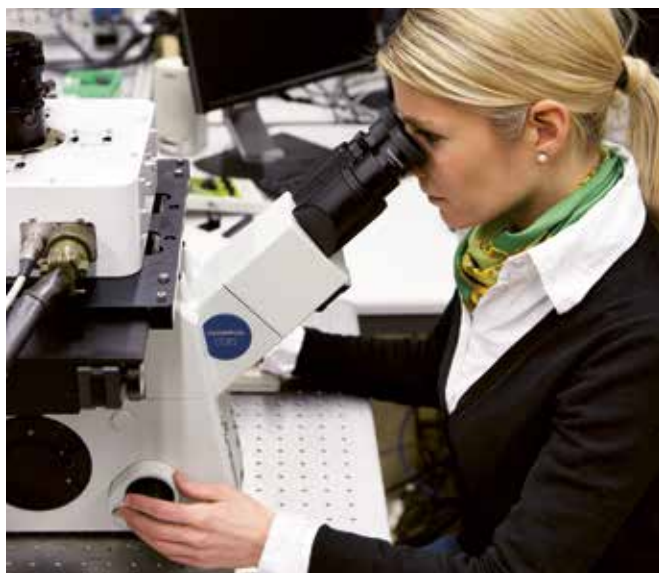
Figure 1: The Nanomag on an inverted microscope for cell manipulation studies
