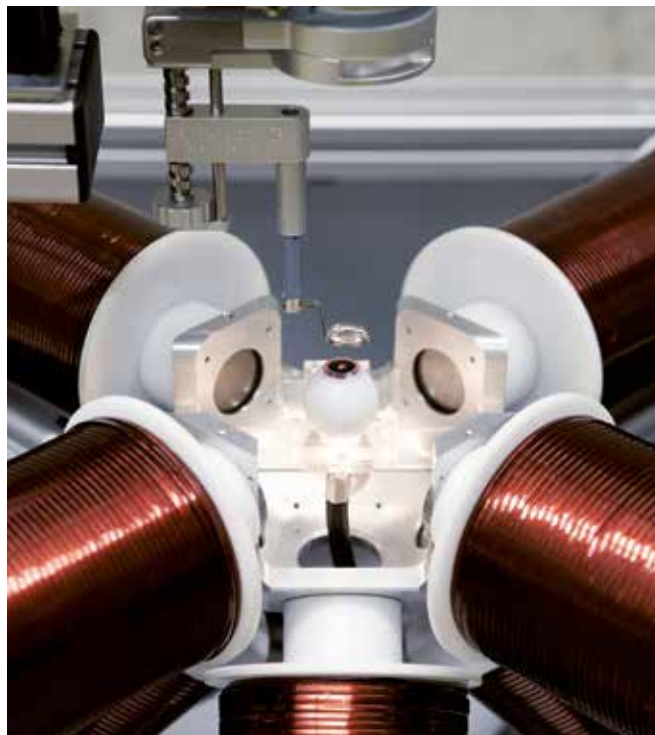
Figure 2: The OctoMag with ophthalmoscope for microrobotic retinal surgery
