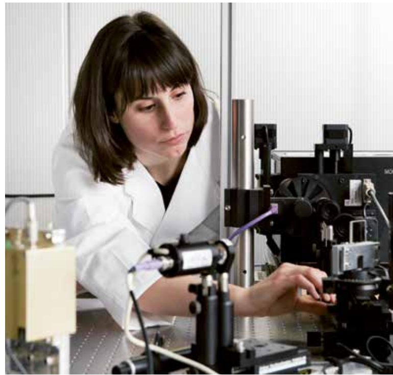
Figure 5: A spectroscopic goniometry system enables the measurement of directional and spectral radiative properties of semi-transparent media, such as complex porous materials applied in thermal and thermochemical energy conversion processes.
