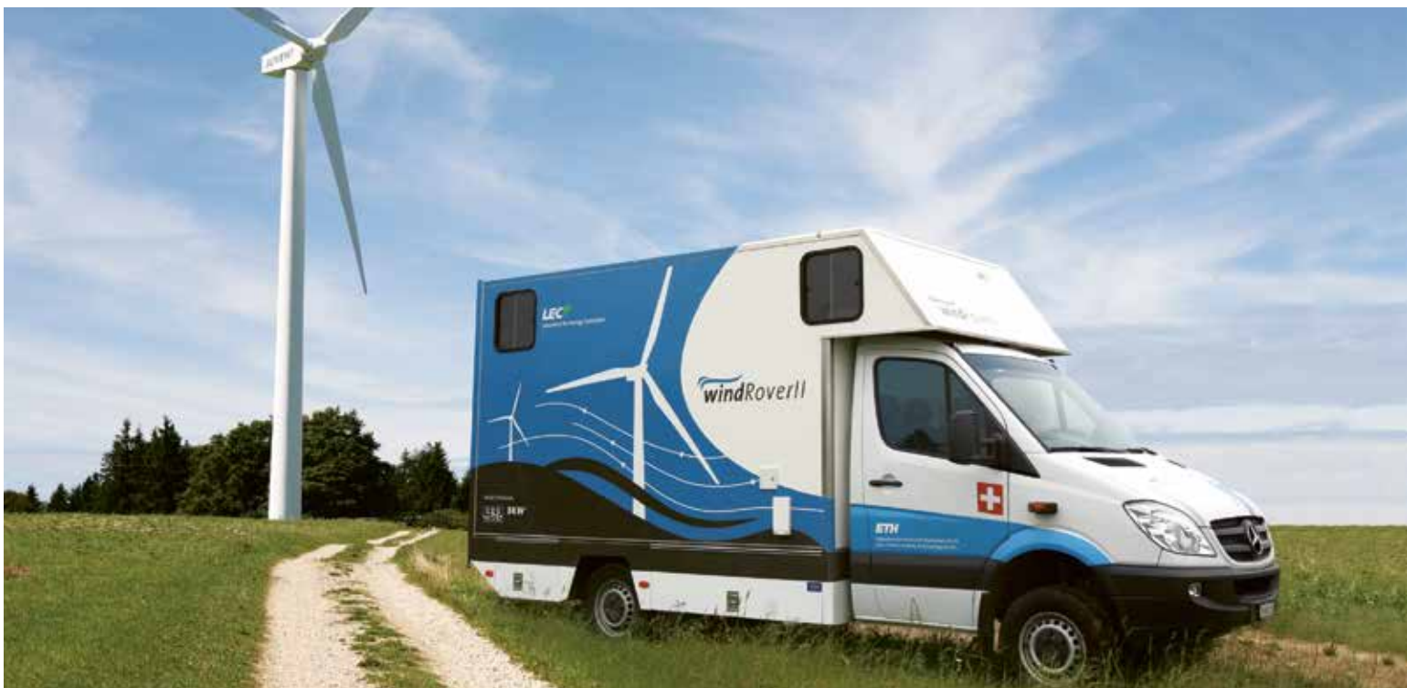
Figure 3: Mobile laboratory equipped with 3D scanning LIDAR system
