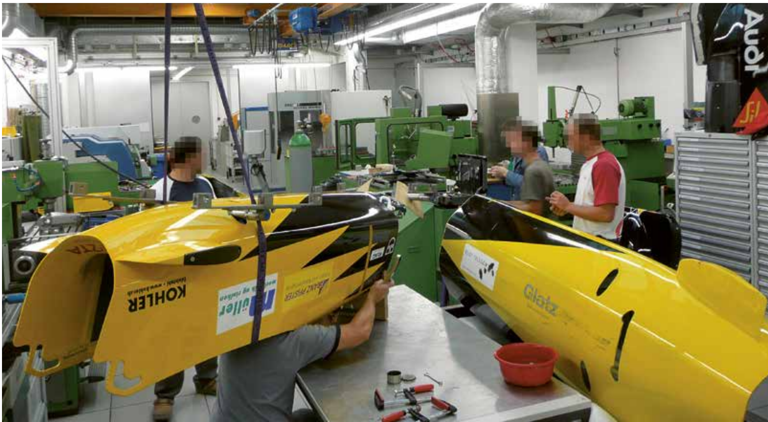
Figure 3: Assembly of the CITIUS bobsleds in the workshop at ETH Höggerberg
