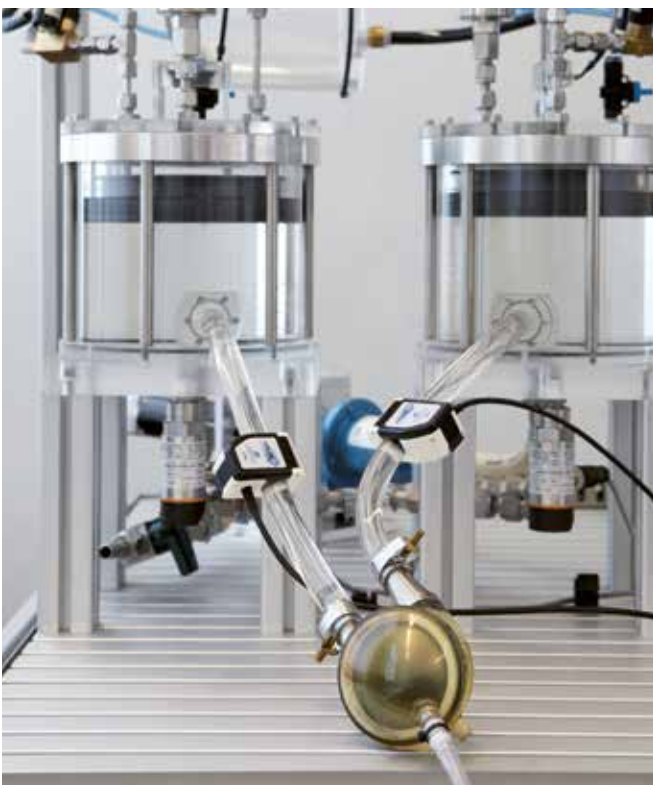
Figure 2: Ventricular assist device testbench
