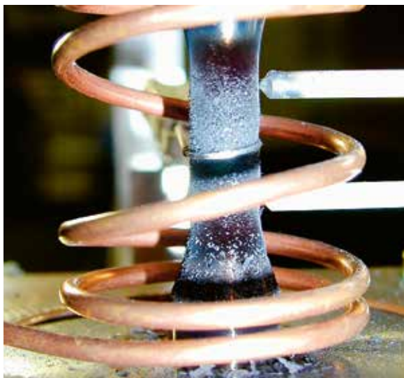
Set-up for service-like thermomechanical fatigue experiments
