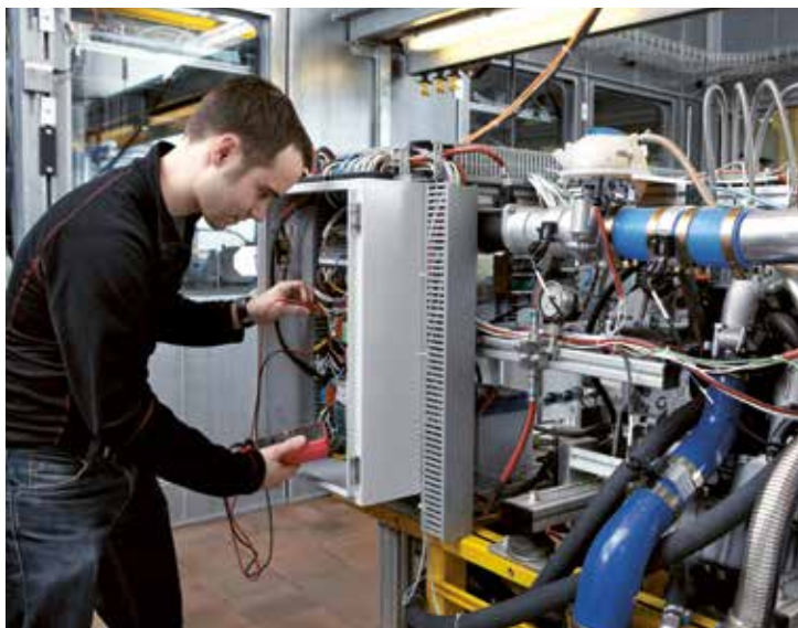
Figure 1: High efficiency CNG engine with diesel pilot injection
