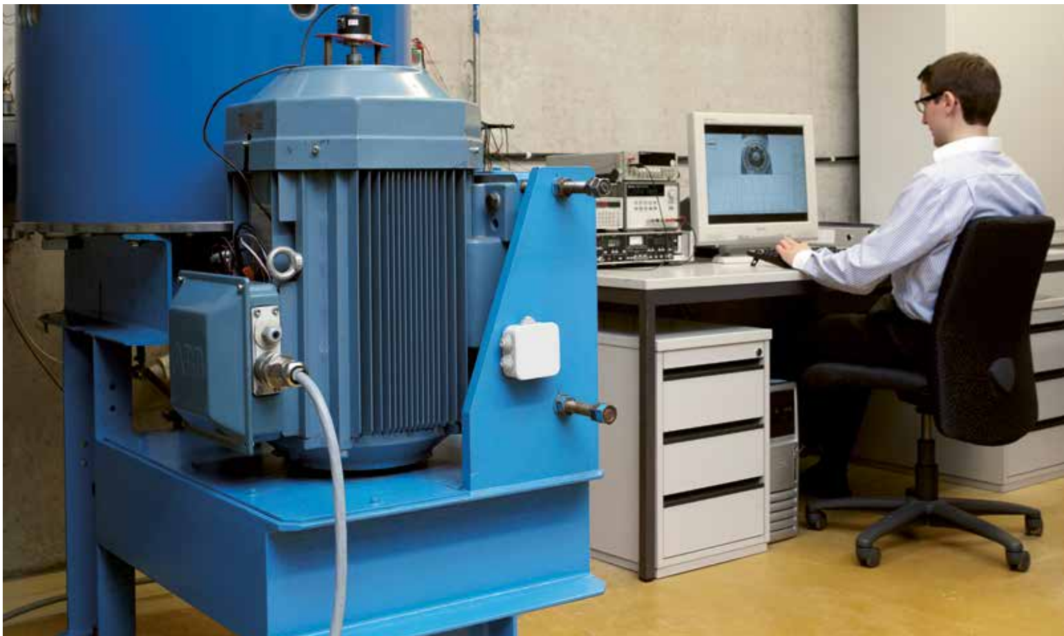
Figure 5: Test facility for the investigation of fluid structure interaction in water turbines
