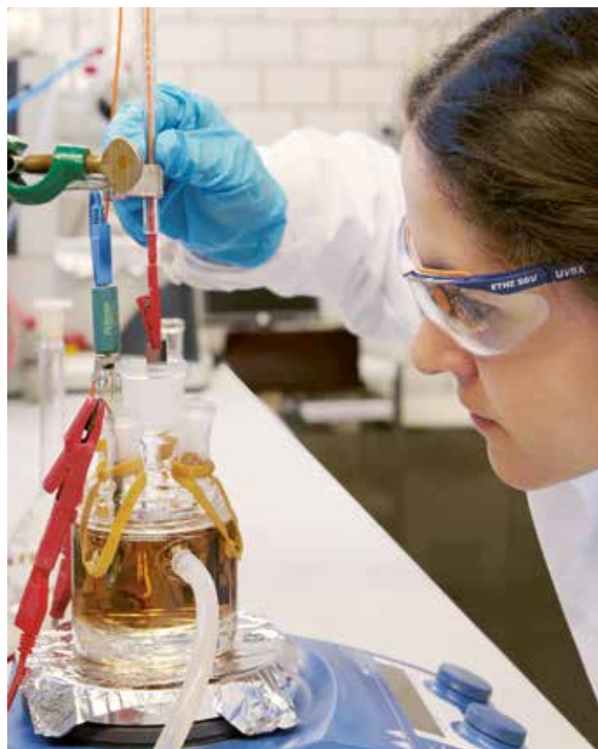
Figure 4: Electrochemical setup to synthesize magnetic patterns of microrobots
