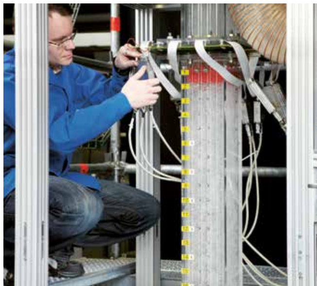
Figure 1: Doctoral student running experiments on coolant cross-mixing and two-phase flow in an adiabatic fuel rod bundle model located at PSI
