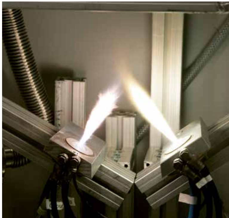
Figure 6: Twin-flame synthesis of Pt/Ba/Al 2 O 3 catalysts for NO x storage-reduction
