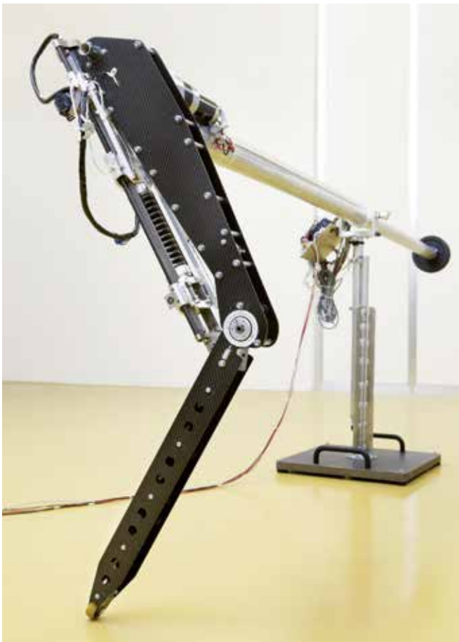
Figure 3: Single leg hopping robot equipped with unconventional actuators
