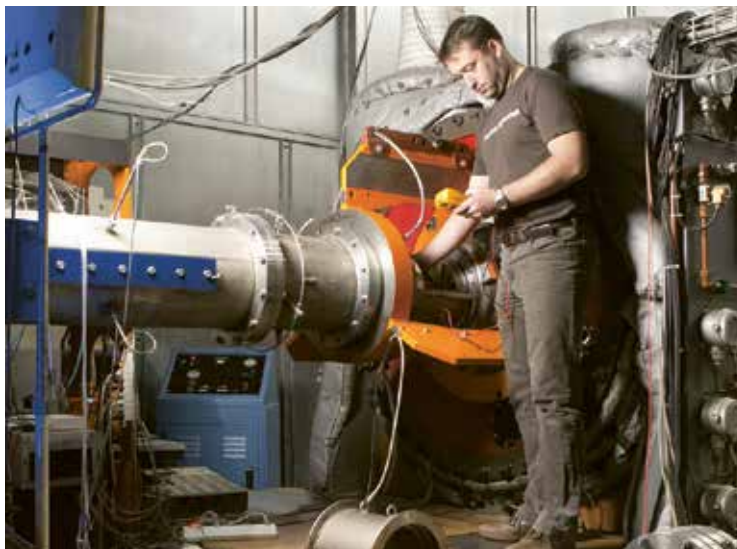
Figure 2: High-speed radial compressor
