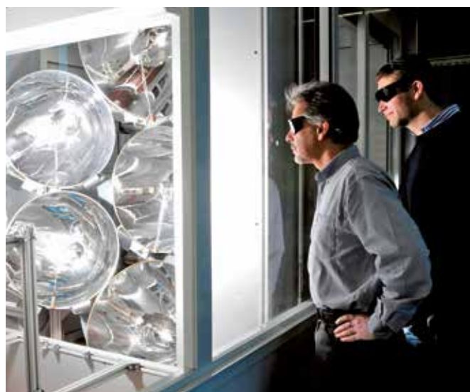
Figure 1: Experimentation at the High-Flux Solar Simulator: solar receivers and reactors are tested at high temperatures (> 1000 °C) and high heating rates (> 1000 °C/s) under similar radiative heat transfer characteristics of highly concentrating solar systems.
