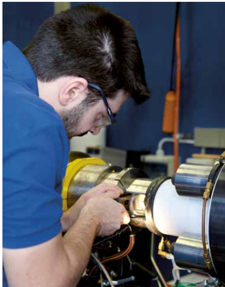
Figure 3: Assembling the optically accessible Rapid-Compression-Expansion Machine
