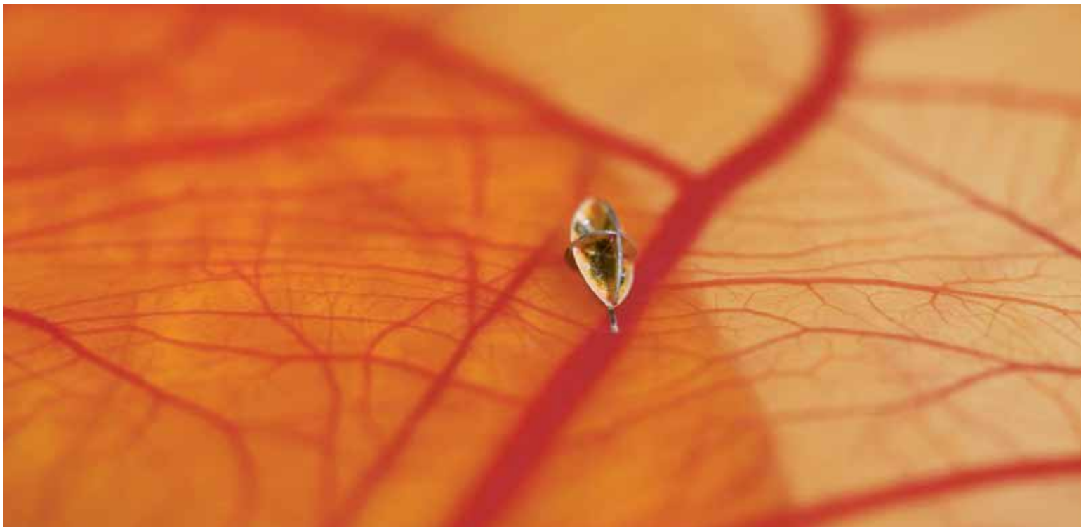
Figure 5: A microrobot docked in a retinal vein model
