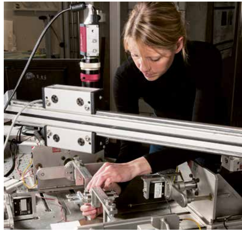
Figure 6: Mounting a mesh implant testpiece in the biaxial machine
