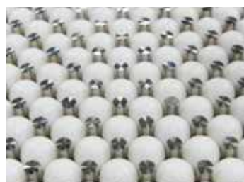
Figure 3: Granular crystals in 1-D (sphere diameter ~200 microns), 2-D (spheres diameter ~1 cm) and 3-D (spheres diameter ~2 mm).
