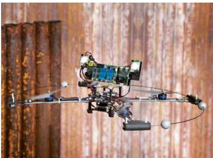
Figure 2: AiRobots: a UAV designed for stereo-camera-based boiler inspection
