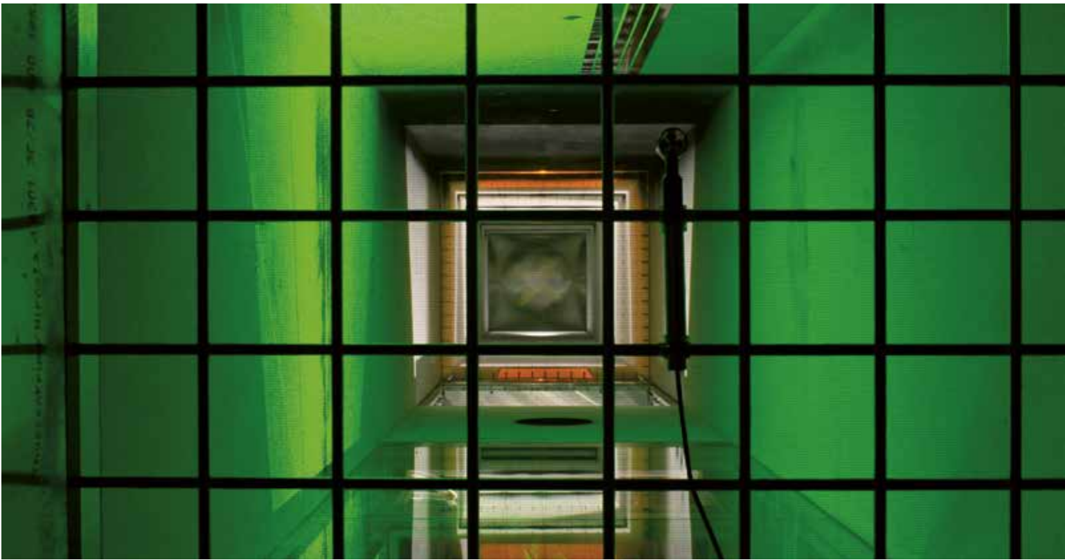
Figure 5: IFD Tunnel Fire Simulation Facility: Study of hot gas propagation using speckle Schlieren imaging and fast temperature grid sensor arrays.
