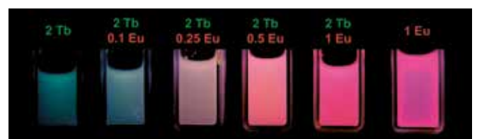
Figure 3: Phosphorescent Eu/Tb-doped \text{Y}_2\text{O}_3 nanoparticles, about 30 nm in diameter
