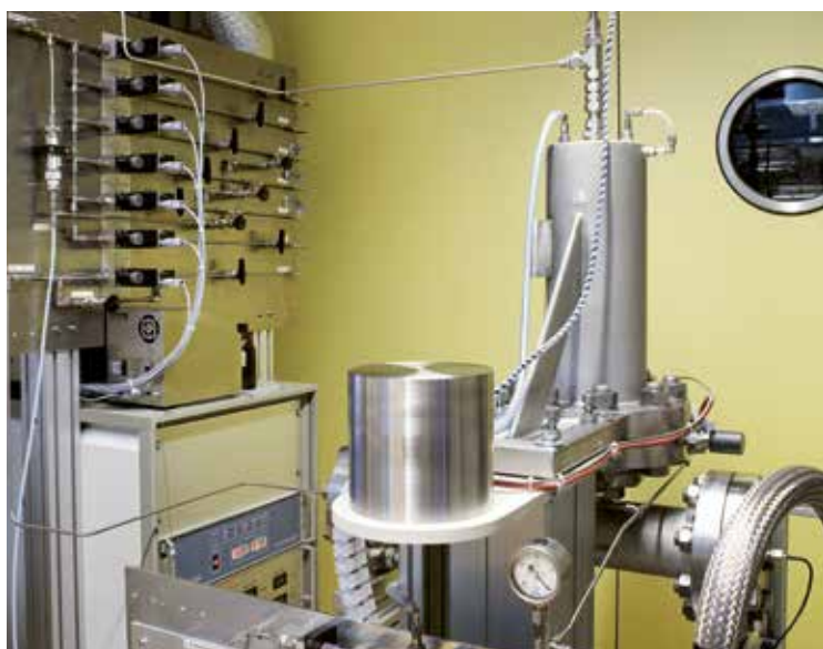
Figure 2: Material characterisation: High-pressure thermo-gravimetric analyser
