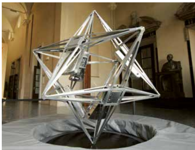
Figure 1: The Balancing Cube is a research testbed used for the development and testing of distributed control algorithms.
