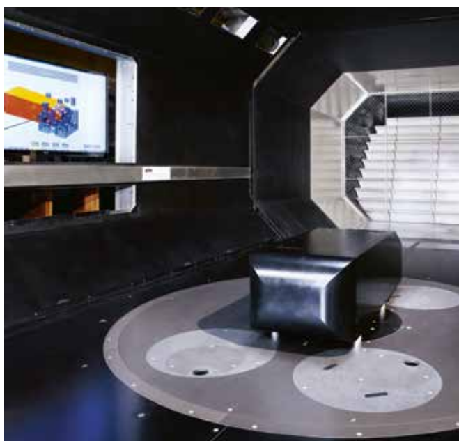
Figure 4: View of the test section in the large IFD wind canal
