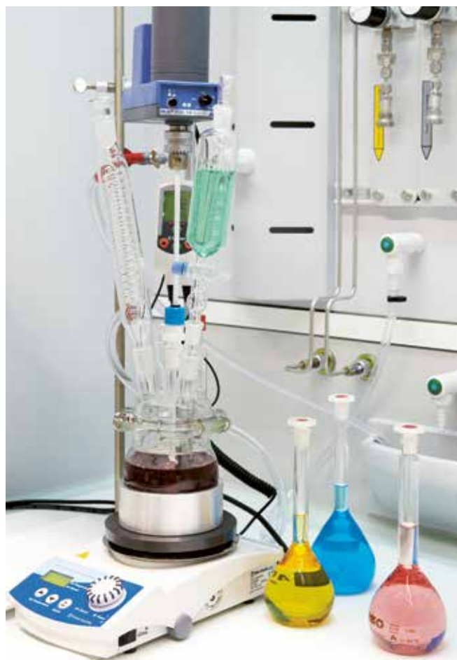
Figure 4: Wet-chemical synthesis of CO 2 sorbents and catalysts
