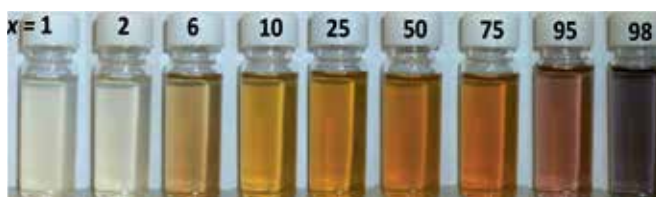
Figure 2: Nanosilver (4 to 16 nm) suspensions with the corresponding plasmonic colors
