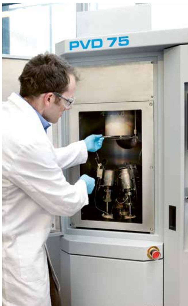
Figure 1: Deposition of metals for the fabrication of plasmonic films
