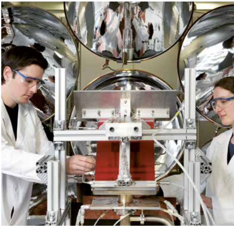
Figure 4: The solar-driven thermogravimeter enables the analysis of reaction kinetics during direct exposure to concentrated irradiation. Gas product composition is monitored on-line by gas chromatography and mass spectrometry. Solid products are characterized by X-ray diffractometry and scanning electron microscopy.
