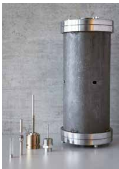
Figure 1: Large and small viscosity sensors: the vibrational characteristics are changed by a fluid interacting with the vibrating structure
