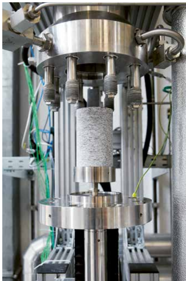
Figure 3: High-pressure vessel for spallation drilling experiments
