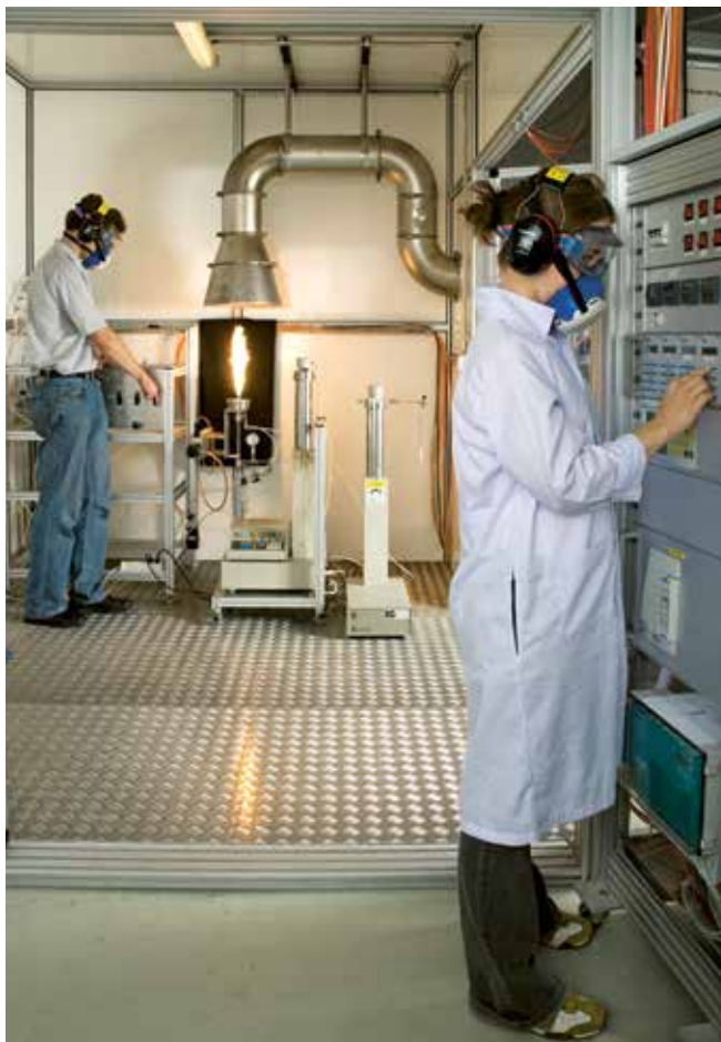
Figure 1: Manufacturing of up to 5 kg/h of ceramic, nutritional and other nanoparticles
