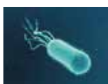
Figure 6: The microrobotic platform called the Artificial Bacterial Flagellum (ABF) was inspired by the swimming technique exhibited by flagellated E. coli .
