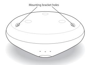
4 Feed the cables through the mounting bracket and then connect them to the base station.
