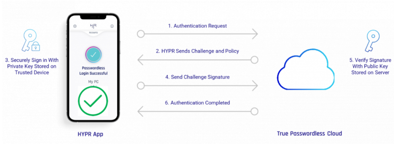
Figure 1: The HYPR authentication flow is initiated from the smartphone [Provided by HYPR]
