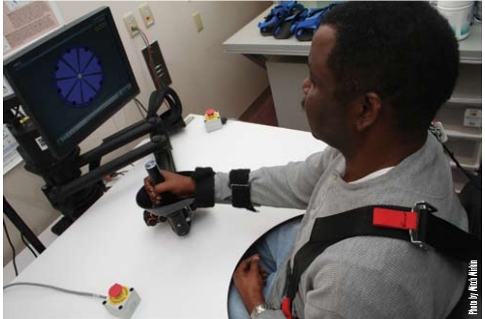
Stroke patient Benson Belo uses a robot called the MIT-Manus at the Baltimore VA Medical Center. The system allows for high-intensity therapy that helps restore strength and function to stroke-affected limbs.
