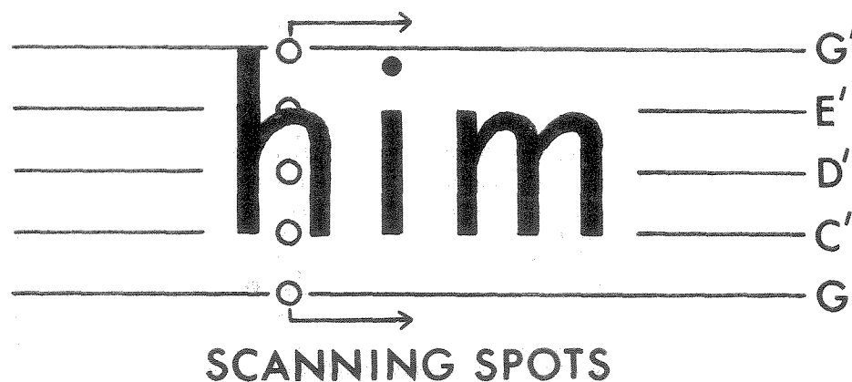
FIGURE 1 Tone generating method of the black-reading Optophone.
