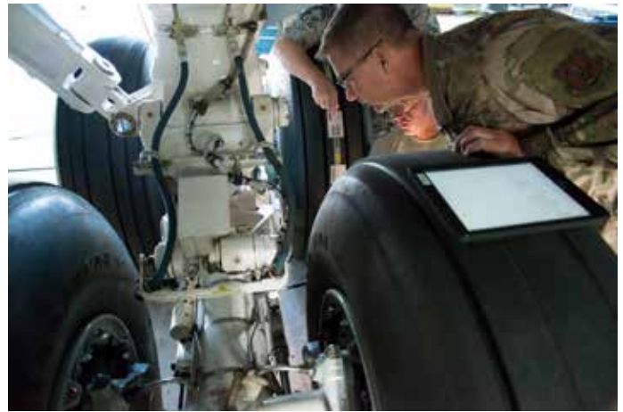
Master Sgt. Jason Stevens, Master Sgt. Tony Garr and Master Sgt. Hal Havens inspect the new centering enior cylinder after a successful test fit, Aug. 15, 2019.
