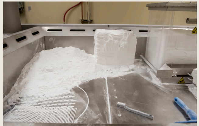
The part cake (left) after being removed from the plastic container on the right. The swabs are inside the part cake. They are made by bonding the nylon powder together one layer at a time using a precisely controlled laser machine.
