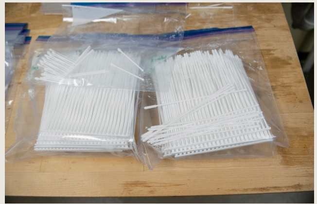
The swabs once they have been separated from the powder and cleaned. They are bagged in lots. Samples are removed to undergo engineering tests and for traceability in case of an unforeseen problem. The bags are then sent for further cleaning and sterilization, after which the swabs are put in a sealed sterile bag and labeled for VA inventory.
