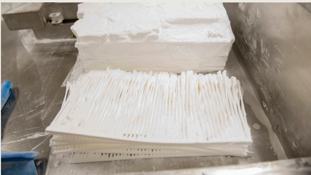
Swabs removed from part cake (front) but not yet cleaned. In the rear is the part cake removed from its container, but with swabs still within the unbound powder. The process is a bit like that of archeologists separating dinosaur bones from the soil where they are buried. The swabs need to be carefully removed from the part cake powder, just like the bones are carefully removed from the soil.
