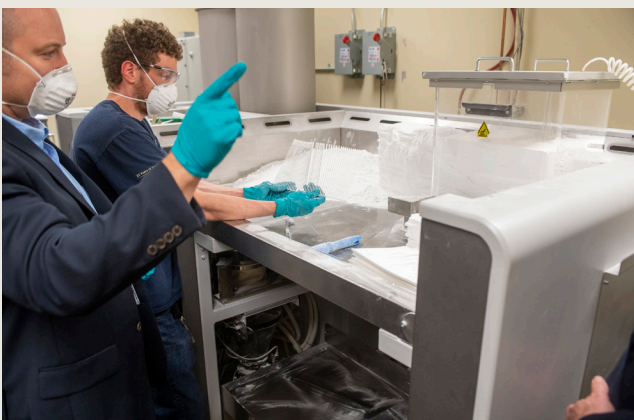
HERL technician Ian Eckstein (R) and Dr. Garrett Grindle, the associate director of engineering at HERL, at the station where 3D-printed swabs are broken-out of the part cake after cooling in an oxygen-free chamber.
