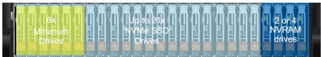
Figure 5. PowerStore base enclosure with drives (front view)
