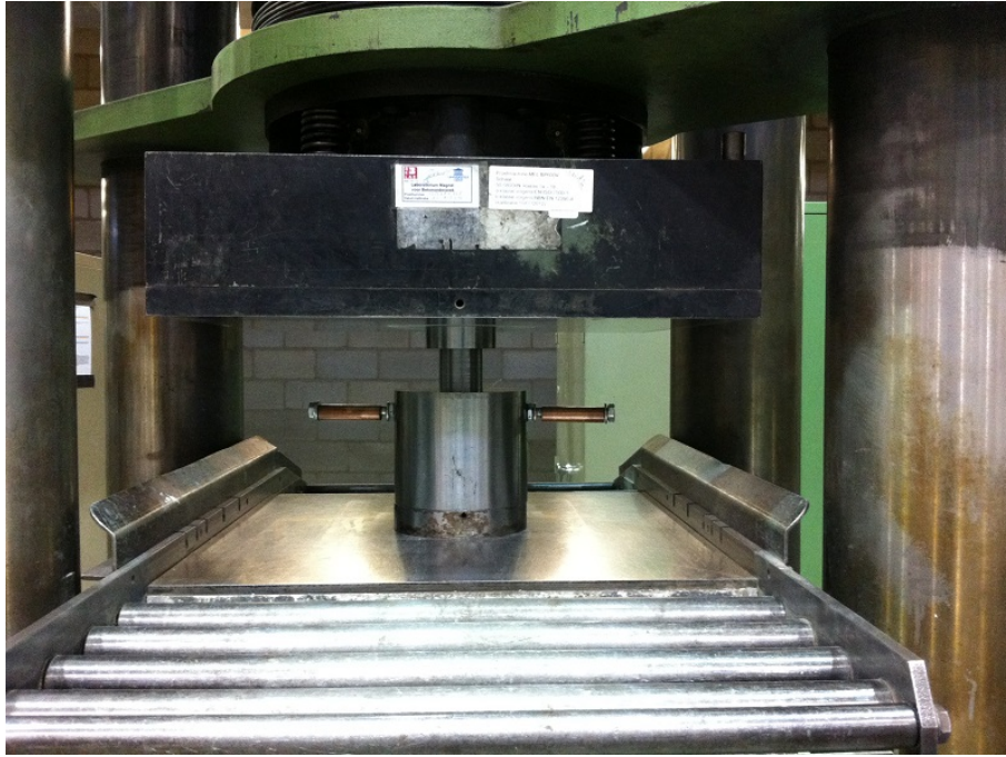
Figure 5.1: The device to extract pore solution of hardened cement paste.
