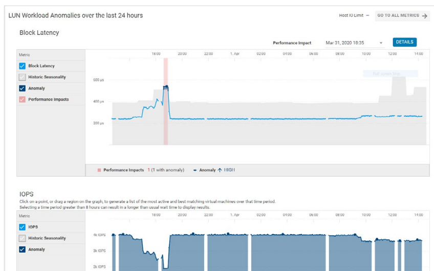
Figure 5: The CloudIQ dashboard showing performance impacts caused by an increase in latency and a drop in IOPS. Source: Principled Technologies.
