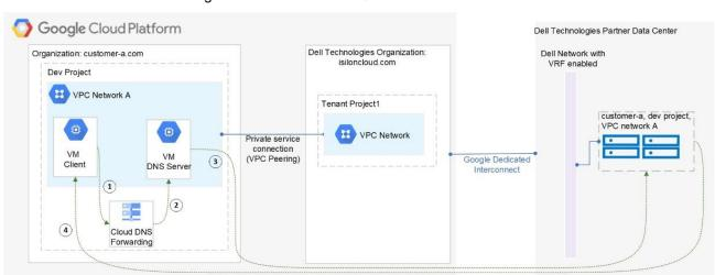
4. SmartConnect returns a node IP to the client. The client can access the cluster data through the cluster service FQDN.
