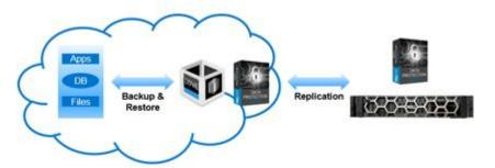
DDVE enables data protection in the cloud for applications running in the cloud. DDVE in the cloud allows for both backup and replication. Data can be moved to an on-premise DD series and backup to the cloud, or even backup and replicate data between two instances of DDVE running in the cloud or on-premise. This allows multiple DDVE instances to be spun up in other regions and backup and replicate the data over to keep everything consistent.
