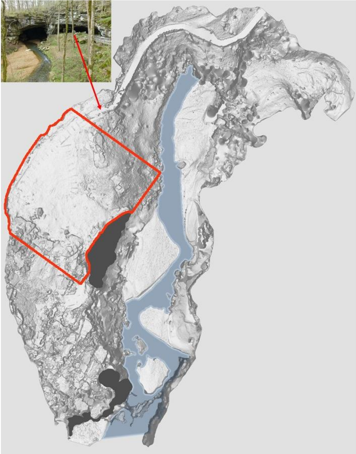
Figure 20. Area of examination for the survey, note that both sides of the cave's rock shelter and surrounding environ were captured with the TLS survey, but emphasis is placed on the dry portion of the shelter for this project.
