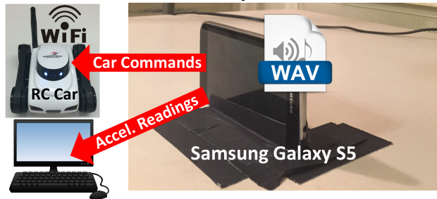
Figure 13. Smartphone Attacking its own Accelerometer to Control an RC Car. An Android phone runs an application that controls an RC car based on the phone’s orientation, measured by its internal MEMS accelerometer. Simultaneously, a malicious audio file is playing over the phone’s speaker, mounting an output control attack on the phone’s accelerometer. The RC car is essentially piloted by the audio file.
