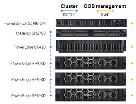
Figure 3: Hardware configuration
