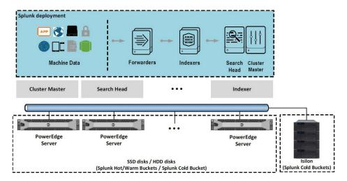
This architecture provides high performance and low latency I/O by using solid-state drive (SSD) storage for Splunk hot/warm bucket data. It also provides high capacity by using hard disk drives (HDDs) or Isilon storage for Splunk cold bucket data.
