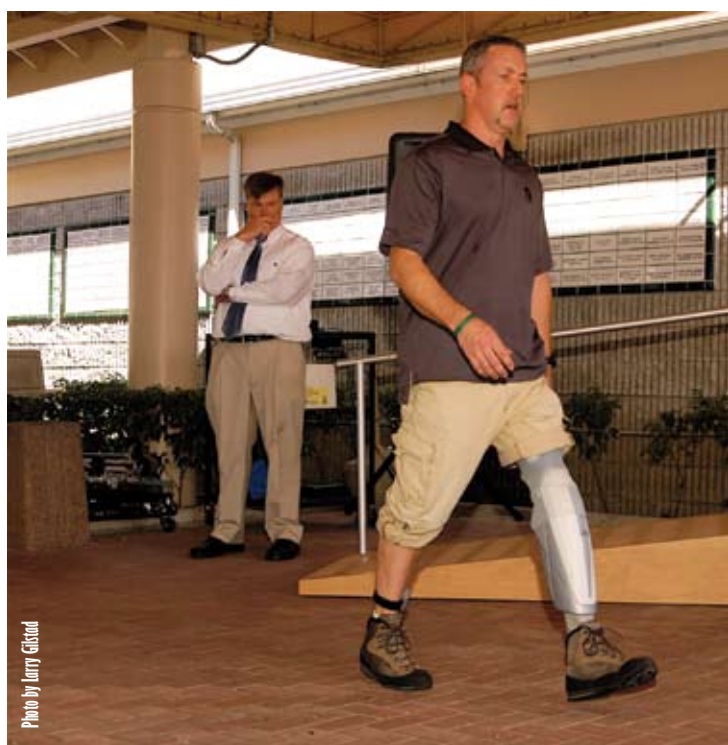
Brad Holling, a Special Forces Ranger who lost his leg when his Blackhawk helicopter went down in Somalia, wears a Power Knee. Part of the system is the transponder on his right leg, which monitors the natural leg’s movement and signals the artificial knee to behave similarly.
