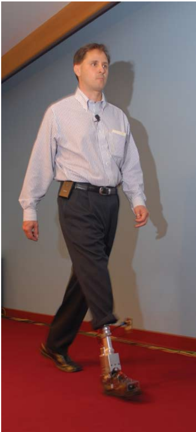
Hugh Herr, PhD, the inventor of the Powered Ankle-Foot and himself a double below-the-knee amputee, demonstrates the device at the Providence VA Medical Center.
