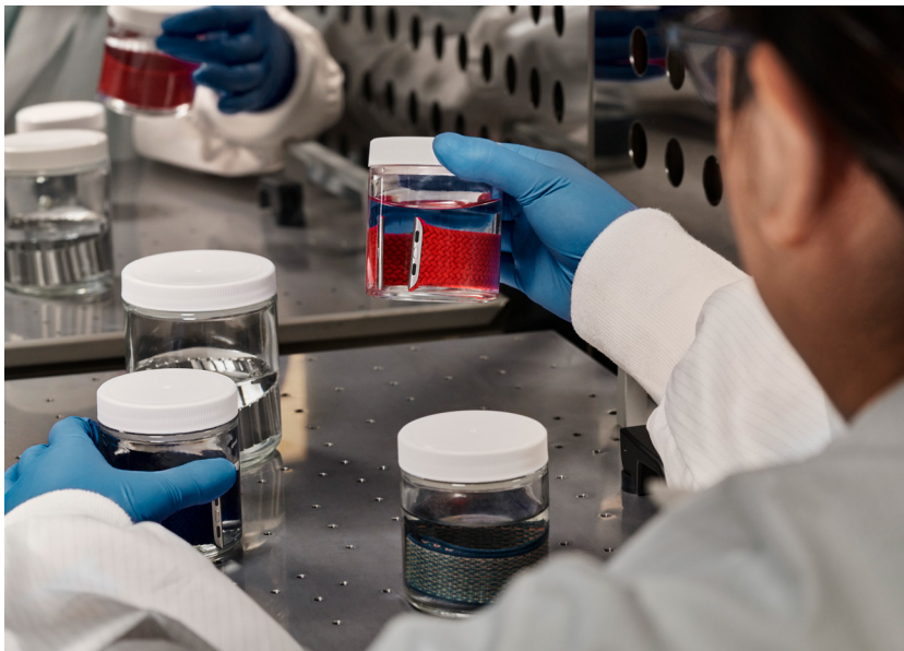
We test products in liquids mimicking sweat to evaluate for biocompatibility.
