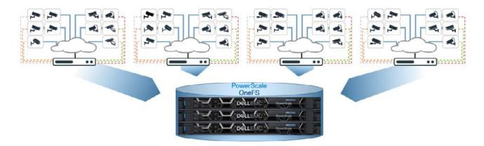
Figure 5: Safety and security system deployment with a PowerScale scale-out NAS system
