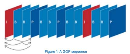
The camera manufacturer's implementation of H.264 causes a video stream's bandwidth to vary over time with changes in the scene. Given the same camera and different scenes shot in different light, the video bandwidth varies from 10 percent to 50 percent, making it difficult to predict the average network bandwidth of a camera's video stream. Streaming video from safety and security cameras represents a highly variable, high-volume data flow.
