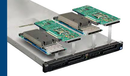
Tejeda cites as one example the BittWare TeraBox 1400DN, which is built on the Dell EMC PowerEdge C4140 server. Working directly with Dell Technologies (product engineers, assisted by OEM Solutions), his team completely re-engineered the server's chassis design to keep its 1U form factor but provide four networking interfaces on its front.
