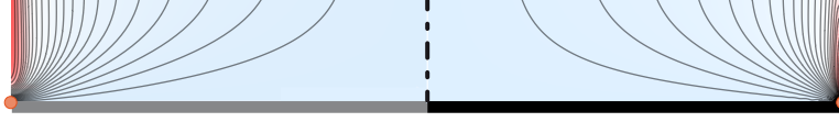
FIGURE 20. Left: Isolines for the radial velocity \tilde{u}_r extracted from the numerical simulations. Right: Theoretical isolines for the radial velocity given by the composite expansion \tilde{u}_r^{\text{comp}} . Note that the transverse scale has here been stretched to visualize the boundary layer.
