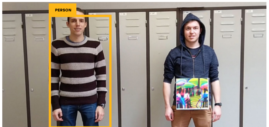
A person detector fooled by an adversarial patch. The illustration from KU Leuven research 2
