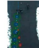
Fig. 1. Comparison of two predicted trajectories in the ETH dataset [1]. CovarianceNet is cyan color, blue and green ellipses, mean, 1 sigma, 3 sigma, respectively. Trajectories+ [2] is yellow stars, yellow and red ellipses, and ellipses+mean, 1 sigma, 3 sigma, respectively. The environment is challenging, since there is a pedestrian in the way.
