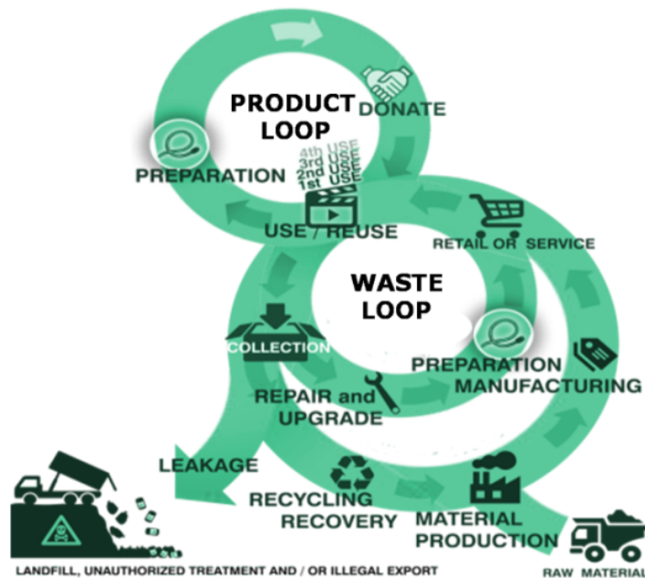
Fig. 1. Main phases and loops on electronics life-cycle
