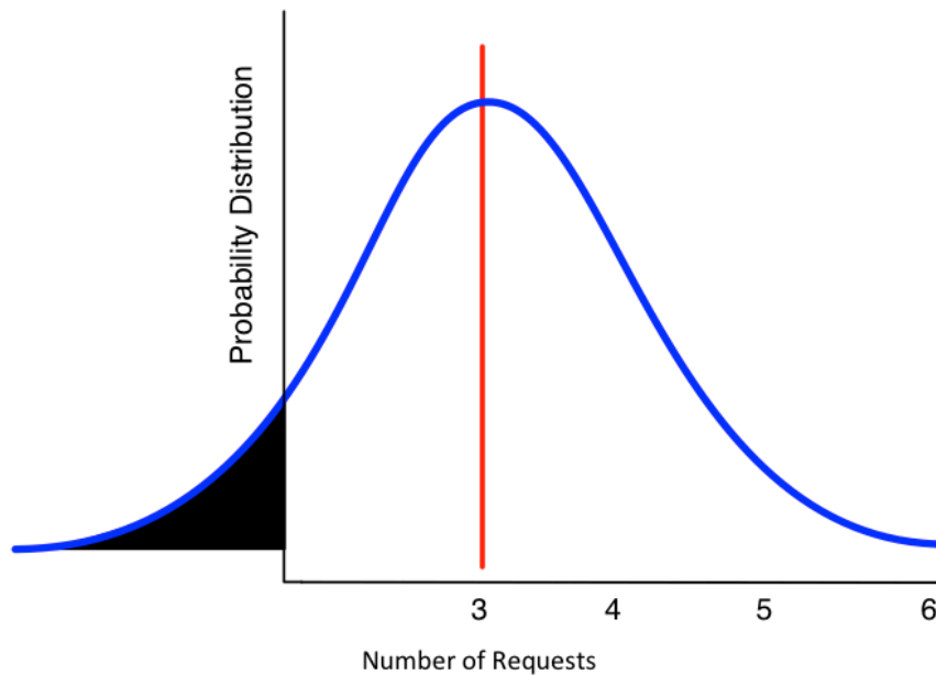
Figure 62 - Truncation errors for Gaussian distributions
