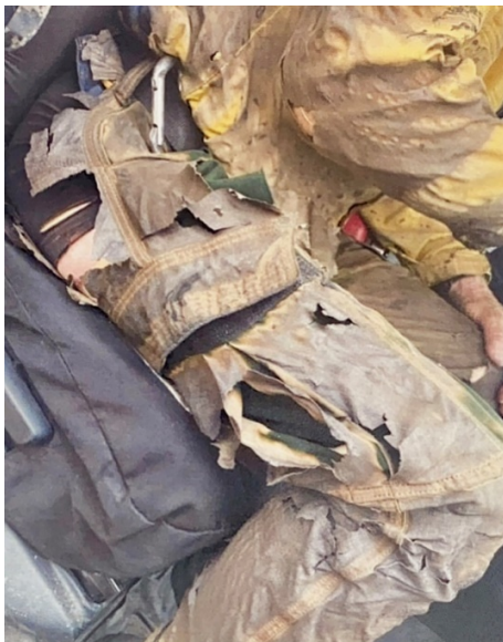
Figure 8. The condition of Dan’s PPE on the right side of his body. These photos were taken shortly after the burnover, prior to relocating Dan from the top of the plateau to the bottom of the hill to wait for EMS.
