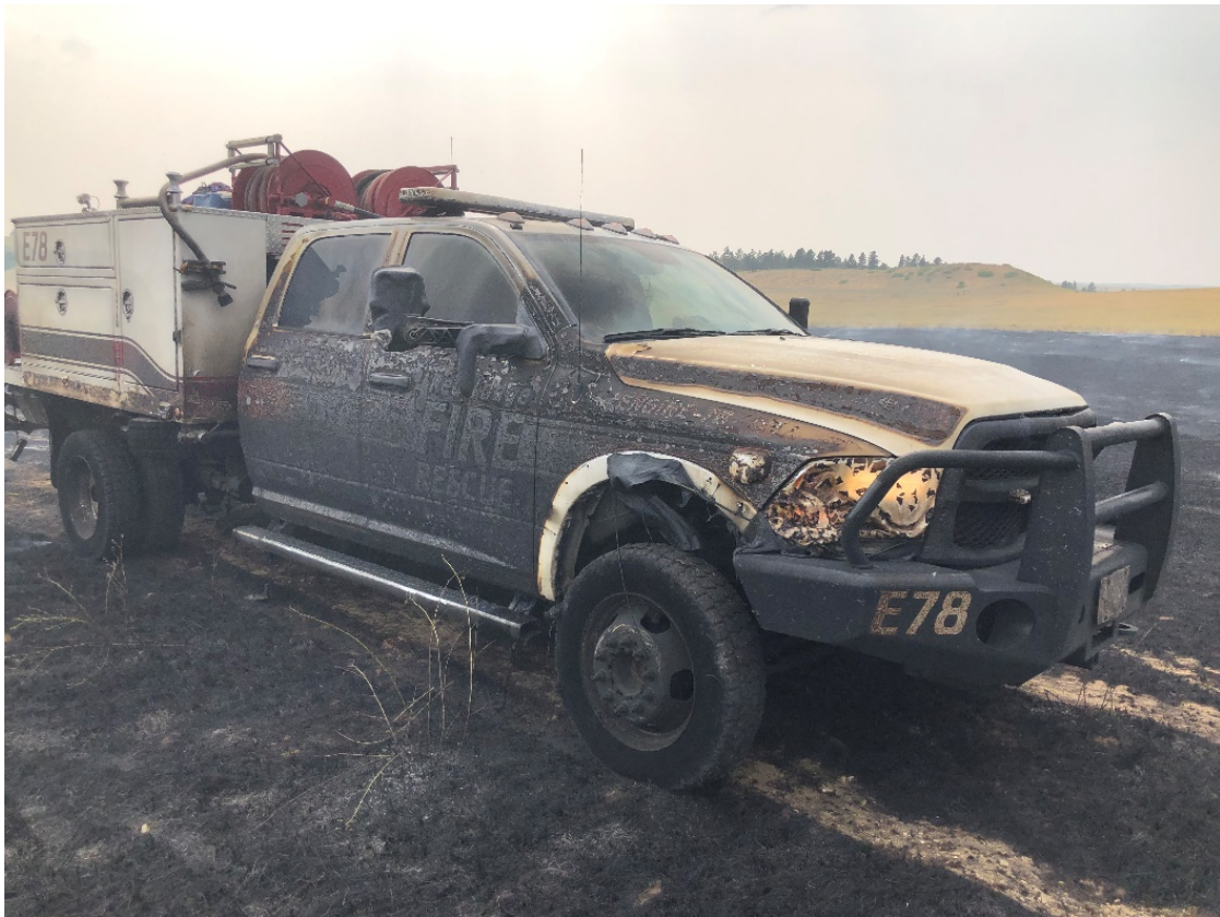
Cover photo: The damage sustained to the Type 6 Fire Engine as a result of the burnover.
