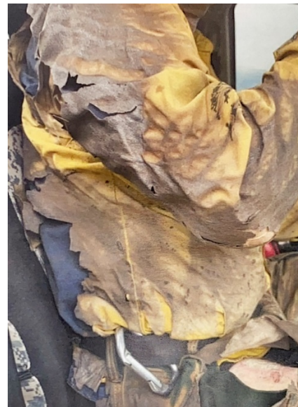
Figure 8. The condition of Dan’s PPE on the right side of his body. These photos were taken shortly after the burnover, prior to relocating Dan from the top of the plateau to the bottom of the hill to wait for EMS.
