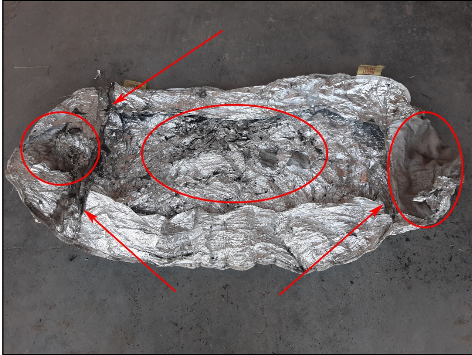
Figure 9: The fire shelter shared by firefighter 2 (FF2) and firefighter 3 (FF3) showing the conditions of the shell inner laminate, floor laminate, and two (2) shake handles. There were several areas where the foil was abraded away, circled in red. Red arrows point to torn floor seams.
