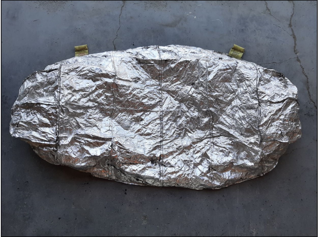
Figure 5: The fire shelter used by firefighter 1 (FF1) showing the conditions of the shell outer laminate and two (2) yellow shake handles.
