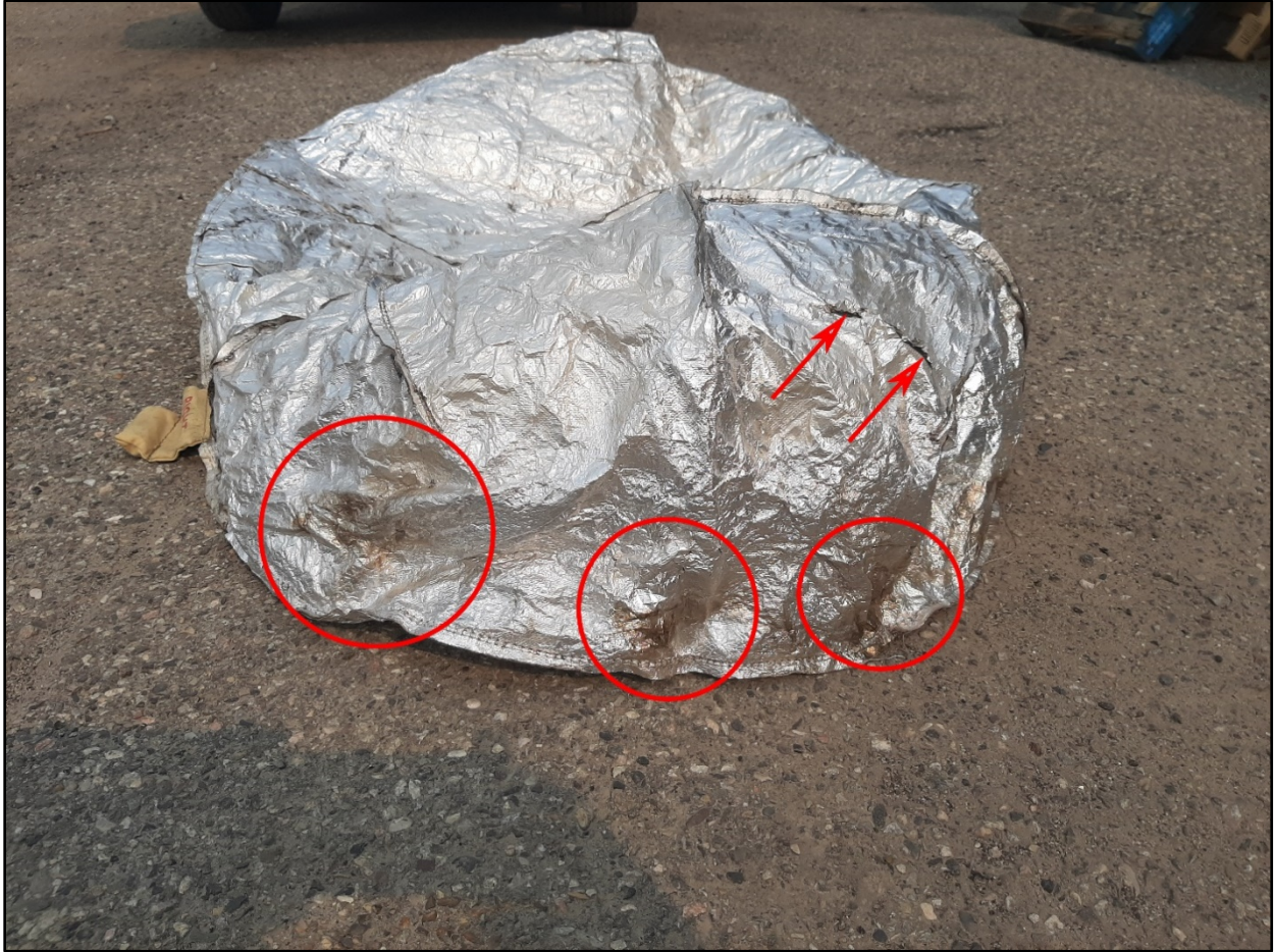
Figure 6: The fire shelter used by firefighter 1 (FF1) showing the conditions of the end cap portion of the shell outer laminate. The foil shows visible signs of heat in three (3) areas that are circled in red. Two (2) red arrows point to the torn foil.
