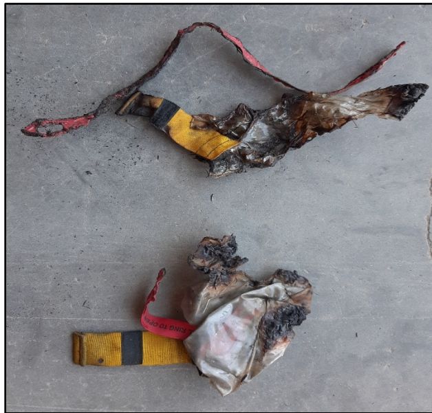
Figure 4: Both polyvinyl chloride (PVC) bags, red pull-tab strips, and yellow nylon pull straps.
