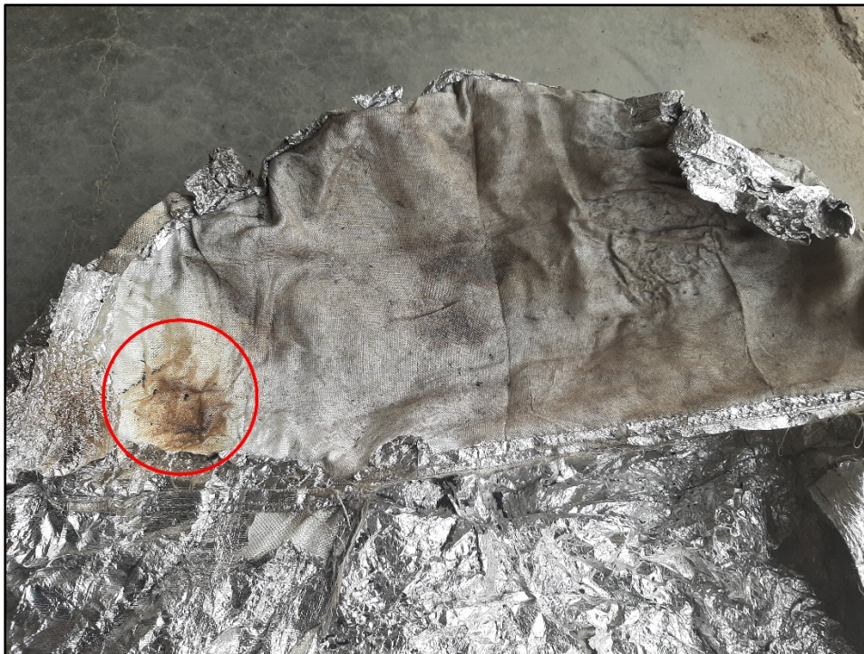
Figure 10: The floor laminate portion of the end cap. The heat-embrittled silica cloth is circled in red.
