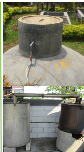
Image: Prototype of biodigester (upper) and biochar furnace (bottom) installation (Source-Balintan).
