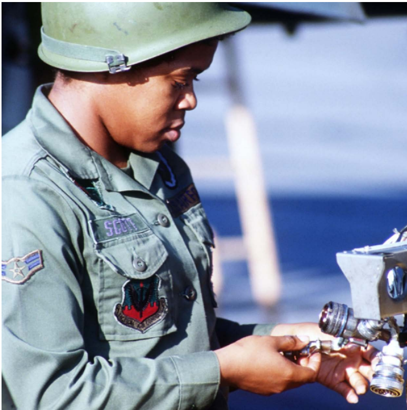
Fig. 16. Airman 1st Class Scott works on an auxiliary power unit that she removed from an A-10 Thunderbolt II aircraft during Exercise Bold Eagle, 1982.
