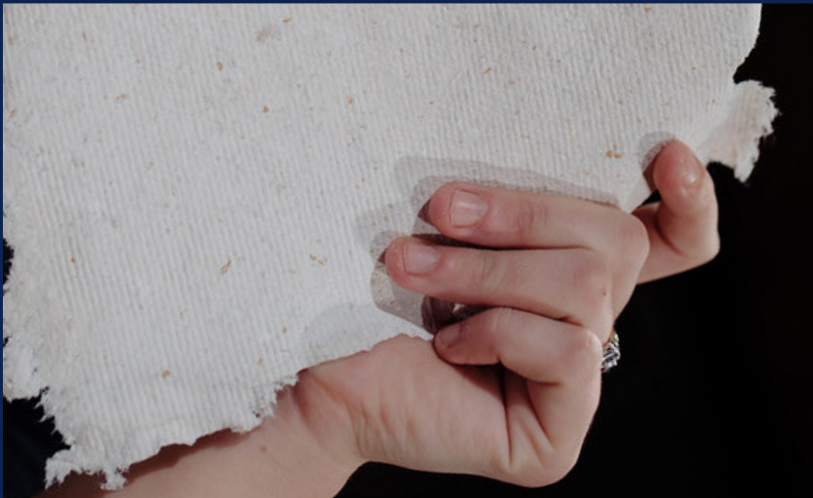
Above: Nonwoven fabrics can be broadly defined as a web of structures bonded together by entangling fibres mechanically, thermally, or chemically. This process bears some resemblance to paper making! Photo by Waag and was retrieved from Flickr in June of 2021.
