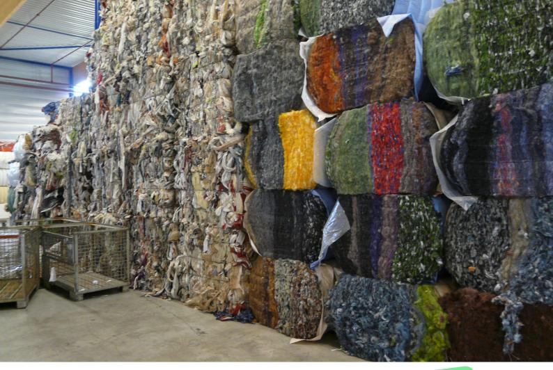
**Above:** Thermoplastic textile waste must be sorted prior to recycling by extrusion. Sorting materials based on colour will result in a more homogeneous colour, but colour variations often occur.
