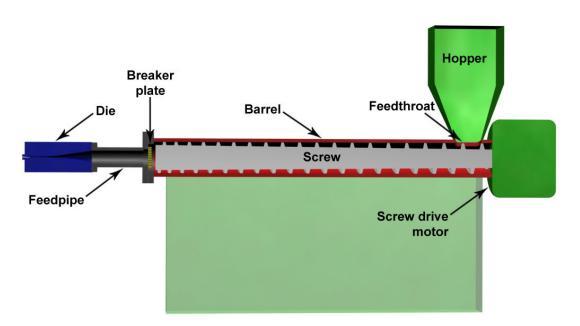
**Above:** A sectional view of a plastic extruder. Plastic granules are melted and then fed into the hopper. The melted plastic is then fed through the barrel and extruded through a die. Photo was released into the public domain by its author and was retrieved from Wikipedia in June of 2020.
