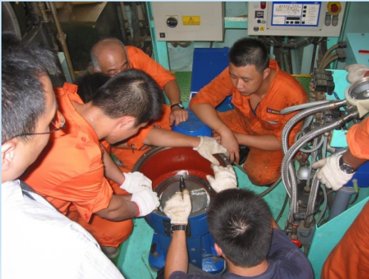
Crewmembers are learning how to reassemble an oil putrefying machine.
