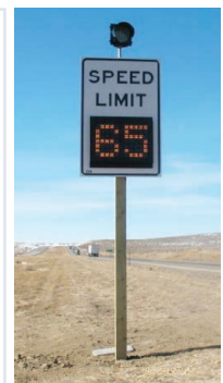
Left: Lead vehicles in truck platoons can save 5 percent of fuel, while following vehicles can save about 10 percent (source: Peloton Technology). Right: Variable speed limit signs can help reduce winter crashes.
