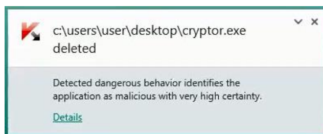
Figure 3. The application is confirmed as malicious, and file that contains the malware is deleted. Affected files stay encrypted
